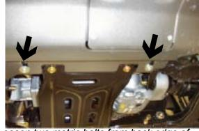
2. Loosen two metric bolts from back edge of belly pan with the 10MM socket, slide belly pan to the back of vehicle to release from slot and set aside.
