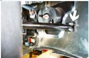
7. Using the 12MM socket, remove metric hex nuts just forward of front tire on the back side of metal bumper, both sides.
