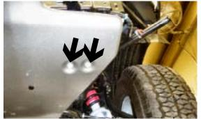
Remove the two torx bolts from belly pan, just below tow hooks with the T-50 torx socket, both sides.
