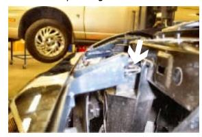
5. Grill tabs will remain in radiator support front. Remove all grill tabs from radiator support and insert grill tabs into back side of grill openings to prepare for reinstallation later.
