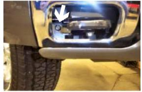
8. Remove the metric bolt from tow hook opening using the 10MM socket, pull metal bumper forward, disconnect all electrical components and set aside.
