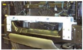
9. Align bolt hole pattern of baseplate to the front of cross member (left photo of passenger's side view), both sides. Install the eight 10MM-1.25 x 35MM hex bolts, lock and flat washers through baseplate, into cross member and tighten. Be sure to use loctite on all bolts before tightening. Tighten all bolts according to Torque Chart in General Instruction Sheet.
