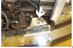
6. Just inside of headlight assembly are two metric bolts to remove with the 12MM socket, both sides.
