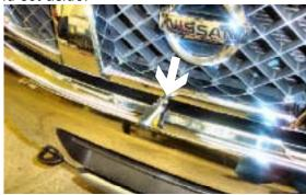
4. Release the three tabs between the lower edge of grill and metal bumper, by inserting flat screw driver into tab slot and rotating screw driver 1/4 of a turn while pulling grill forward to separate grill from tab, set grill face down on a soft surface to prevent scratching.
