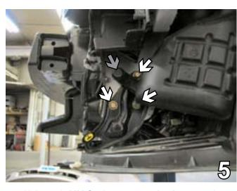
5. Using a 14MM Socket, remove the three metric bolts from the tie-down bracket (see white arrows in photo). This will be done to both sides, the driver's side is shown. On the driver's side remove one bolt from the air baffle using the 10MM Socket (see grey arrow in photo).
