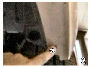
On the underside edge of the front fascia remove two Phillips screws. Set aside to be re-installed later. This will need to be done to both sides of the vehicle, the driver's side is shown.
