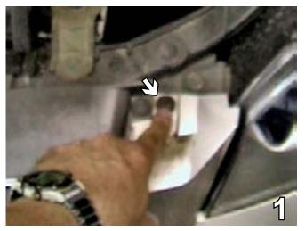
Remove four push pins from the top of the front fascia and set aside to be re-installed later. This is done all along the top of the front fascia, the driver's side is shown.
