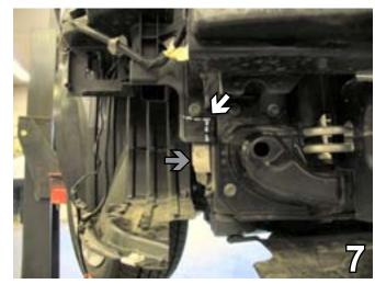
7. Using a reciprocating saw, cut the black plastic under the frame extension bolt horizontally from the outside edge to the frame rail and bend the plastic forward. Finish removing the black plastic by cutting along the bend (white arrow shows trim). The grey arrow shows the webbing which must be bent flush with the frame rail. This is done on both sides of the vehicle, passenger's side is shown.
