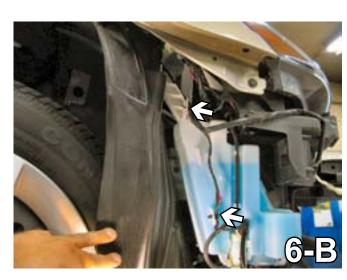
Remove the three metric bolts from the windshield washer reservoir with a 10MM Socket. Release the two wire clips, then disconnect and plug the hose and electrical wires. Set all aside to be reinstalled later.
