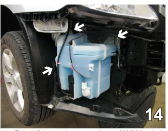
14. Reinstall the washer reservoir, use 30MM hex bolt with five 1/4" flat washers behind each tab.
