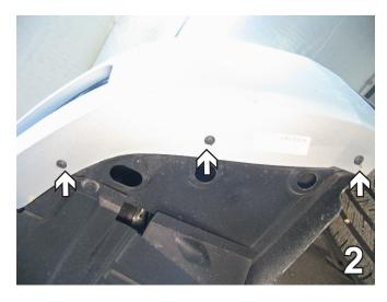
On the underside edge of the front fascia remove three Phillips screws. Set aside to be re-installed later. This will need to be done to both sides of the vehicle, the driver's side is shown.
