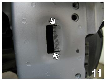
Using a reciprocating saw make a cut at the edge of the opening, bend the metal cut in. Do this on both sides.
