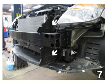
7. Remove the black plastic from above and below the frame extension by pulling it out. This is done on both sides of the vehicle.
