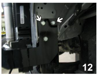
12. Insert 1 1/2" hex bolt and 3/8" lock washer into the top two holes and fasten to a 1" nut plate inserted through the opening on frame end. Use Loctite Red and torque to specifications. Do this on both sides.
