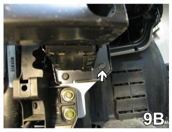
9. Using a 13MM Socket, remove the four metric bolts from around the bumper. Do this on both sides. Remove the bumper and the frame extension, set aside to be reinstalled later.
