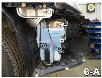
On the passenger side, remove the three metric bolts from the windshield washer reservoir with a 10MM Socket. Release the two wire clips from the electrical wires, then disconnect and plug the hose. Set all aside to be reinstalled later.
