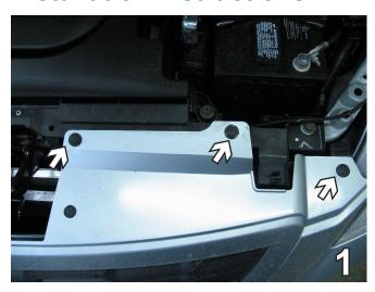
1. Remove three push pins from the top of the front fascia and set aside to be re-installed later. This is done on both sides, the driver's side is shown.
