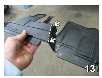
13. Cut the black plastic at the angle shown with a utility knife. Reinsert the top piece.
