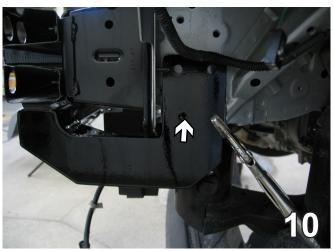
10. Lift the baseplate up and push it as far forward and up as possible. Be sure it is level with the vehicle, clamp with a vise grip. The lower hole should align in the middle of the lower frame webbing. Drill holes into lower hole of baseplate using a 13/32" drill bit. Insert 1 1/2" hex bolt, 3/8" lock washer and 3/8" whiz nut. Use Loctite Red on all bolts. Do this on both sides.
