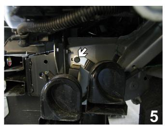
On the driver's side using a 13MM Socket, remove the metric bolt from the horn. Unplug and set aside to be reinstalled later.
