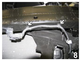
8. Unplug the sensor by pulling the tabs out of the lower bumper.
