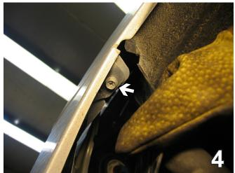
4. Using a 10MM Socket, remove one metric bolt from the inside of the wheel well, just forward of the front tires, and set aside to be re-installed later. This is done on both sides of the vehicle, the driver's side is shown. Pull the fascia corners out to the side of the vehicle, just above the front tire to release, both sides, then pull fascia forward and set aside carefully for later reinstallation.
