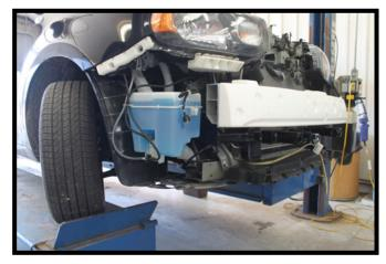
21. Reinstall the plastic shielding, frame extensions, bumper, styrofoam filler and washer reservoir.
