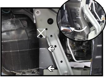
12. On the passenger side, using a reciprocating saw, trim out the upper portion of the frame face and cut two (2) slits back to the frame side. Bend the face back around flush to the frame side.
