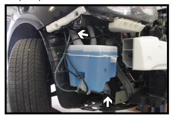
Using a 10MM socket, remove the two
