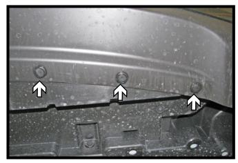
4. Remove the three (3) push pins from the underside front of the fascia. Do this on both sides of the vehicle.
