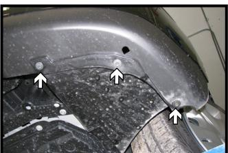
Using a 10MM socket, remove the three
