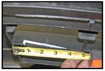
16. On the backside of the fascia, trim the outside of the middle rib. From the outside edge go in 3/4" up 1/2" into the rib. Then over 3" tapering off flush. Do this on both ends of the fascia.
