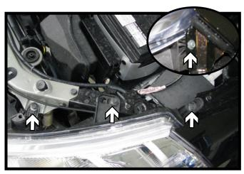
Using a 10MM socket, remove the three
