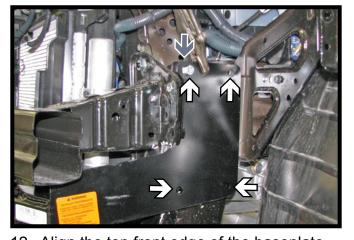
12. Align the top front edge of the baseplate with the top of the frame rail (gray) and pull the baseplate as far forward as possible. The top back edge of baseplate will dip slightly below the top of the frame rail. Level and clamp the baseplate into position. Using the baseplate as a template to drill four (4) 13/32" holes (white) into the frame rail. Do this to both sides of the vehicle.
