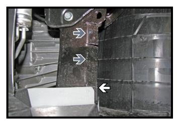
11. Using a reciprocating saw, cut the lower portion of webbing where it begins to angle down (white) to the webbing of the frame rail. Flatten the sections (above this cut, not below it) flush against the frame rail (gray) with a hammer. Do this to both sides of the vehicle.
