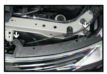
Remove the two (2) push pins from the top of the fascia. Do this on both sides of the vehicle.
