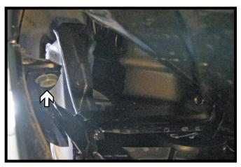
5. Pull the wheel well cover back, then using a 10MM socket, remove the screw from the inside top edge of the fascia. Do this on both sides of the vehicle. Remove the fascia from the vehicle.
