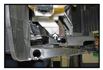
On the passenger side, disconnect and/ or cap the electrical connections and fluid lines from the washer reservoir. Using a 10MM socket remove the lower bolt.
