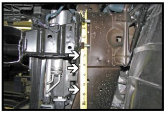
10. Mark the frame rail webbing at 5", 6-1/2" and 8-3/4" from the top of the frame rail. Using a reciprocating saw, cut the webbing to the frame rail (the top cut goes through bumper bracket also). Cut and remove the upper section of the webbing. Do this on both sides of the vehicle.
