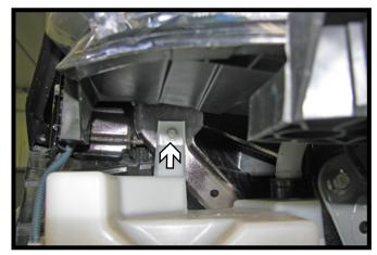
8. Using a 10MM socket, remove the upper bolt from the reservoir. Disconnect the filler tube and remove the reservoir from the vehicle.
