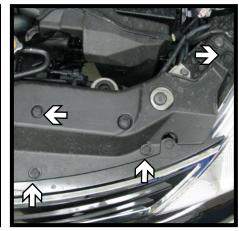
1. Remove the eleven (11) push pins from the top of the radiator cover and remove from the vehicle.
