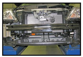
15. Reinstall the washer reservoir and headlights.
