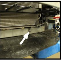
9. Using the existing stud, attach the breakaway bracket and securely fasten with the 8MM x 1.25 nut that has been provided.
