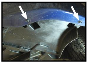
2. Using a 20 torx remove the two (2) screws underneath the vehicle on the outside edge. Towards the center there are three (3) push pins that need to be removed. Do this on **BOTH** sides of the vehicle.
