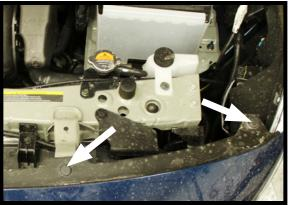
Remove the five (5) push pins that are located in the front area, underneath the hood. There are two (2) push pins located on the outer edges on **BOTH** the driver side and the passenger side. There is also one (1) located in the center.
