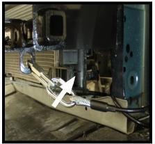
the baseplate. The photo above shows the recommended installation of the cables to frame of vehicle. Additional options may interfere with suggested mounting; in this case, secure the cables to a solid piece of the frame as described in the instructions included with the permanent baseplate safety cables. Be sure the safety cables do not rub against any hoses or moving parts. Do this on **BOTH** sides of the vehicle.
