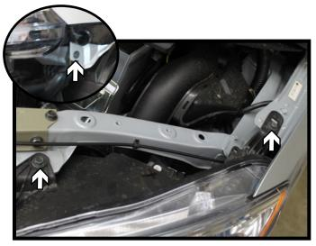
Using a 10MM socket, remove the two
