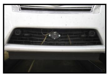
17. Hold the fascia as close to its original position, mark and trim the fascia around the convenience links and attachment tabs. Reinstall the washer reservoir, air baffle, headlights, metal bumper, styrofoam, fascia and fascia cover.
