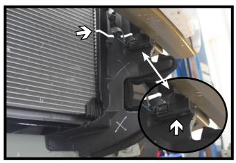
On the driver side, remove the temperature sensor from the shrouding (inset). Then trim off the lower section of the shrouding flush with the bottom of the bumper.
