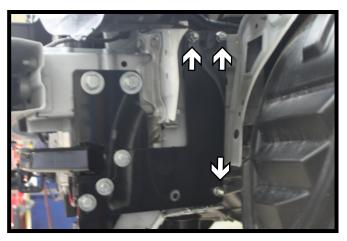
16. Using a 13/32" drill bit, drill the three (3) support plate holes thru the frame. Install 3/8"-16 x 1-1/2" bolts with 3/8" lock washers and nuts on the inside of the frame. Do this on both sides of the vehicle.
