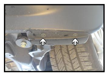
4. Using a 10MM socket, remove the four (4) screws from the underside of the fascia in front of the tire. There are two (2) on each side.
