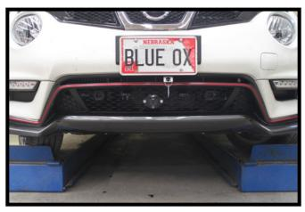
19. Hold the fascia as close to its original position, mark and trim the fascia around the convenience links and attachment tabs. Reinstall the washer reservoir using the supplied lower bolt. Reinstall the baffle and fascia.
