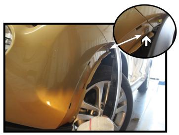
Gently pry the fender flare away from the vehicle. Using a 10MM socket, remove the exposed screw at the fascia and fender seam. Do this on both sides of the vehicle.
