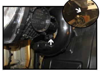
6. On the driver side, using a 10MM socket, remove the screw from the lower section of the baffle. Remove the push pin from the upper section just below the blinker (inset). Set the baffle aside.
