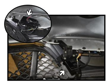
18. Nismo Only: On the backside of the fascia, unscrew the fog light box and flip upside down and reattach to the fascia as shown for baseplate clearance. Do this on both sides of the fascia.
