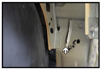
12. Using a hammer, flatten the ridge behind the frame webbing. Do this on both sides of the vehicle.
