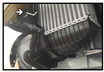
On the passenger side, trim the lower section of the shrouding off flush with the bottom of the bumper.
