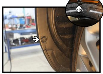
2. In the wheel well, remove the two (2) push pins. There is one (1) on the lower edge and one (1) on the upper edge (inset). Do this on both sides of the vehicle.
