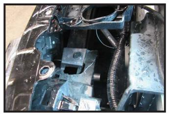
4. Remove the push pin from the inner fascia. Do this for both sides of the vehicle.
