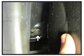
11. Using a 10MM socket, remove the three (3) screws from the air baffle. There are two (2) on the front top, and one (1) on the backside, between the wheel well cover and the baffle.
