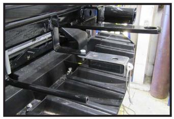
**Optional Breakaway:** Bolt the breakaway to the baseplate bracket with the supplied 1/4" hardware.
