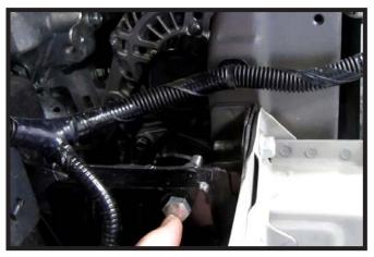
17. Drill one (1) 3/8" hole and start a 3/8" x 2" bolt with a flat washer and nylon lock nut on the back.
