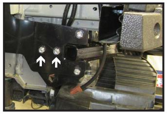
23. On the passenger side install the remaining two (2) 3/8" x 1-1/4" bolts with nylon lock nuts on the back.
