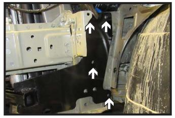
20. On the driver side of the vehicle start drilling the four (4) 3/8" holes need for the bracket. Start with the top two (2) holes, then drill the bottom hole, and finally drill the middle hole. Make sure the bracket stays level while drilling each hole.
