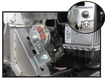
12. Using a 10MM socket remove the horn and horn bracket from the passenger side to be reinstalled later.
