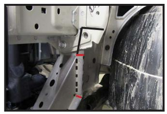
14. On the driver side use a reciprocating saw to cut along the marked area (black) across and down. Then make two (2) slots (red) as indicated Use a hammer to bend the piece forward along the dotted line.
