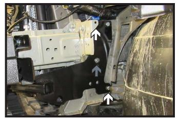
22. On the driver side install the two (2) remaining 3/8"-16 x 1-1/4" Hex Head bolts with a flat washer and nylon lock nut on the back as indicated (white). Then insert one (1) 3/8"-16 x 1-1/2" Hex Head bolt and a Whiz nut with 14" wire on the back (gray).
