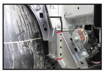
On the passenger side use a reciprocating saw to cut along the marked area (black) across and down. Then make two (2) slots (red) as indicated. Using a hammer bend the piece forward along the dotted line.
