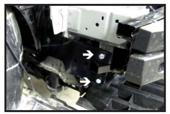
19. Start two (2) 3/8" x 1-1/4" bolts with nylon lock nuts on the back on the passenger side.
