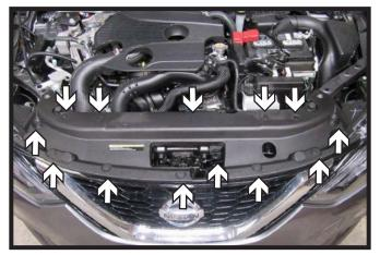
1. Remove thirteen (13) push pins from the fascia cover. Remove fascia cover and set aside.
