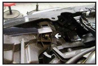
3. Using a flat screwdriver, push in the pictured clip, and pop the plastic piece out. Do this for both sides of the vehicle.
