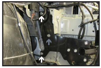
24. On the passenger side insert the two (2) remaining 3/8"-16 x 1-1/4" Hex Head bolts with a flat washer and nylon lock nut on the back as indicated (white). Then insert one (1) 3/8"-16 x 1-1/2" Hex Head bolt and a Whiz nut with 14" wire on the back (gray).
