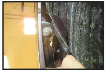
6. Using a 10MM socket, remove the bolt from behind the wheel well cover where the fascia meets the fender. Do this on both sides of the vehicle.
