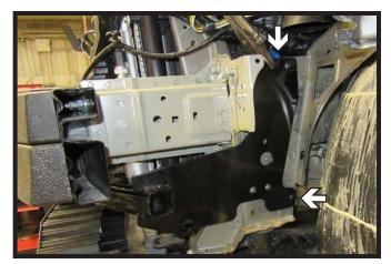
Attach cross member so that the driver side plate is level at the top of the frame and flush with the bottom back piece as indicated. Use vise grip to hold into place.
