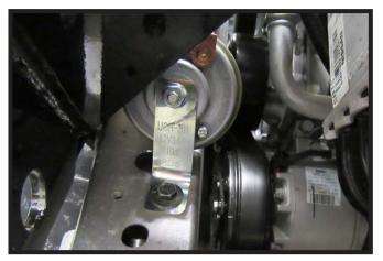
25. Bend the horn bracket to allow for baseplate clearance and reattach the horn as indicated.
