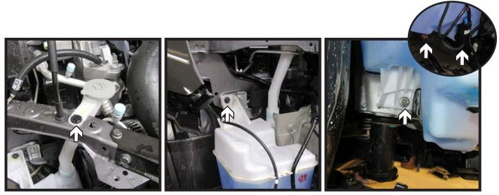
10. Remove the one (1) push pin from the top of the windshield wiper fluid reservoir. Using a 10MM socket, remove the one (1) bolt from the upper front of the reservoir, and the one (1) bolt on the back side of the reservoir. Unplug the two (2) connections from the front of the reservoir, plug the fluid lines, and remove the reservoir.
