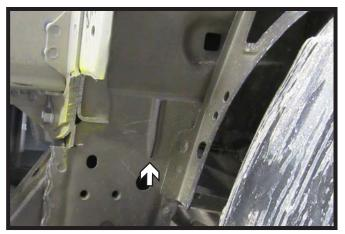
15. Using a hammer flatten out the indicated piece so that it will not interfere with the baseplate. Do this for both sides of the vehicle.
