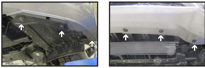
5. Using 10MM socket, underneath the fascia, remove three (3) bolts. Next, remove three (3) push pins. Do this for both sides of the vehicle.
