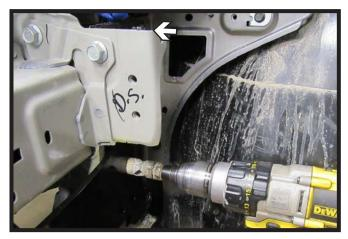
21. On the driver side start a 3/8"-16 x 1-1/4" Hex Head bolt with the flat washer and nylon lock nut on the back in one (1) of the top drilled holes. Then using a 1" hole saw drill out the center access hole, do this on both sides of the vehicle.
