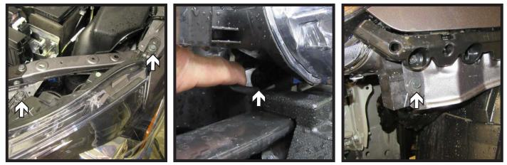
9. Using a 10MM socket, remove four (4) bolts, with two (2) on top, one (1) below, and one (1) on the side. Disconnect the wiring, remove headlights and set aside. Do this for both sides of the vehicle.
