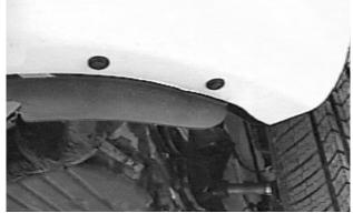
6. Remove the push pins from the bottom of the bumper fascia. Pull off the bumper fascia from the vehicle and set aside. Remove the rock guard connected to the lower cross member.
