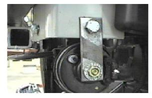
14. Reinstall horn using bracket provided, item9. Be sure to use loctite on all bolts before
