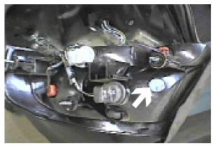
**Note:** If installing the BX8869 bulb and socket wiring kit, this is the recommended location for drilling the hole.
