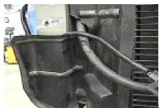
**6.** Remove two push pins on the air dam, both sides and set aside.
