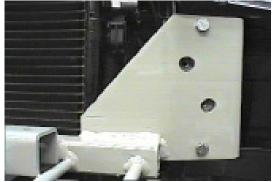
**9.** Hold baseplate in place so that top edge of end plates are flush with top frame webbing. Using the baseplate as a template, drill four holes on the front side of baseplate with the 13/32 drill bit. Insert items 3, 4, and 5, do not tighten.
