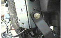
7. Unplug electrical connection from horn and remove horn bracket with a 10MM socket, then set aside. Factory horn bracket will not be reused.
