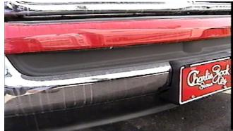
For a vehicle without tow hooks has a plastic trim piece that will need to be removed. Once this is removed, bolt the baseplate to existing holes in frame with 1/2-13 x 1 1/2 hex bolts, lockwashers and hex nuts as shown on page 2(items 2, 3 and 4). Be sure and use loctite on all bolts before tightening. Tighten and torque all bolts according to chart on the General Instruction Sheet.
