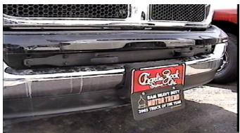
**1.** For a vehicle with tow hooks, remove the six 15MM bolts to remove the tow hooks. Using existing metric bolts and fasten the baseplate to the truck. Be sure and use loctite on all bolts before tightening. Tighten and torque all bolts according to chart on the General Instruction Sheet.
