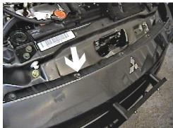
Using the 10MM socket, remove the five metric bolts from the top side of front fascia.
