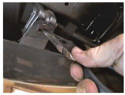
**5.** Using the needle nose pliers, remove one center-clip push pin on the bottom, middle of fascia, pull pin down and set aside.
