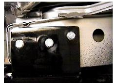
11. While maintaining a level position with the bottom of frame, hold spacer plate up as far as possible and 1/4" back from frame end. Using spacer plate as a template, drill holes with the 13/32" drill bit, both sides.
