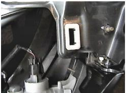
Just behind headlight assembly is one metric bolts to remove with the 10MM socket, both sides.
