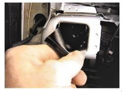
**12.** Insert backing plate into frame end to align with drilled holes, both sides.
