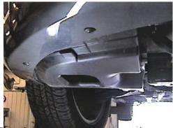
4. Forward of front tires remove three push pins on wheel well edge and three on the bottom edge of front fascia, both sides.
