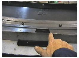
**15.** Lay fascia face down on a soft surface, remove tab just behind license plate bracket and reinstall fascia, trim as needed.
