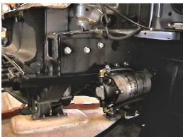
13. Hold baseplate and spacers to align with drilled holes while maintaining a level position with bottom of frame, both sides. Install 3/8" bolts and lock washers on both sides, tighten all bolts. Be sure and use loctite on all bolts before tightening. Tighten all bolts according to torque chart in General Instruction sheet.
