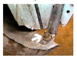
**4.** Just forward of front tire is one metric bolt to remove from metal bumper bracket using the 19MM socket, both sides.
