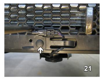
21. The air temperature control will not go back into the original hole. Hold it up and drill another hole.
