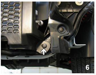
6. Using a flat screwdriver, remove the push pin on each side of the opening under the fascia.
