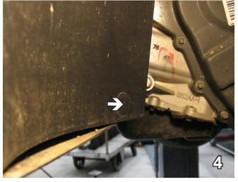
4. On the driver side only, follow the fire wall around to the back, use a flat screwdriver to remove the push pin. Set the pin aside for later reinstallation.
