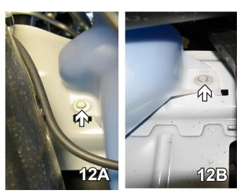
12. Using a 10MM socket, remove the two bolts one on each side of the washer reservoir. Set washer reservoir and bolts aside to be reinstalled later.
