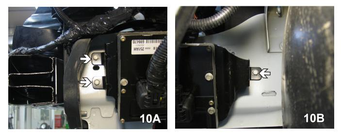
10. On the driver's side, using a 10MM socket remove two bolts on the front and one on the back then let the computer hang down in order to do drilling. Set bolts aside to be reinstalled later.
