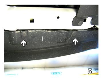
5. Using a flat screwdriver, remove four push pins from underneath the front edge of the fascia. Set push pins aside to be reinstalled later. The corner of the fascia is then pulled out to the side and forward to remove. Set fascia aside carefully to be reinstalled later. Be sure to unplug the fog lights.
