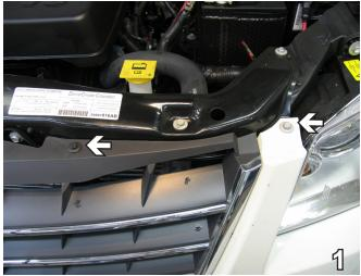
1. Using a 10MM socket remove the bolt above the headlight. Using a flat screwdriver remove the push pin. Do this to both sides and set bolts and push pins aside for later reinstallation.
