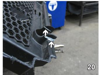
20. On the back side of the plastic shield, cut off the six tabs.
