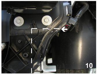
10. Using a utility knife, cut straight across right along side the bottom of the plate and straight up to a 90° angle. Do this on both sides.
