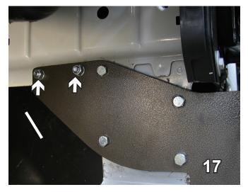
17. On the passenger's side, the top two bolts are brought from the inside out because of the black plastic shield. The same 3/8" x 1 1/4" hex bolts and 3/8" lock washers and 3/8" hex nuts are used. Be sure to use LOCTITE Red on ALL bolts.
