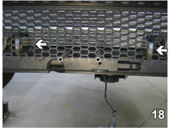
18. Hold the plastic shield up to the front and with the utility knife cut out as needed for the baseplate tabs.
