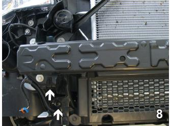
8. Using a flat screwdriver, remove the push pin. Then using a utility knife, cut the loose plastic right along the bumper. Do this to both sides.
