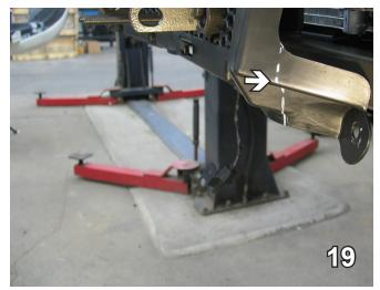
19. Using the utility knife cut 3" straight down on the corner of the plastic shield. Do this on both sides.
