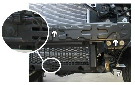
Using a flat screwdriver, remove the push pin from the air temperature control and let it hang (see arrow in inset). Continue removing four more push pins across the top. Remove the plastic cover.
