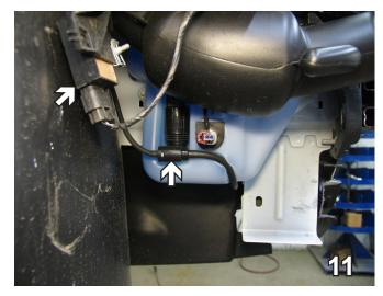
11. Unplug the electrical plug and take the water lines off the washer reservoir and plug them.
