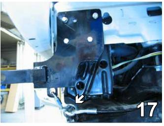
17. Attach the baseplate safety cables. Position the cables around a solid piece of the frame.
