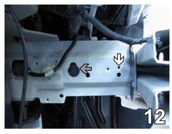
12. On the passenger side, using the 13/32" drill bit, drill another hole in alignment with the washer reservoir existing hole. Also enlarge the existing hole to the back with a 1 1/4" hole saw (gray arrow).
