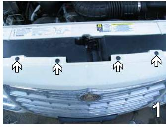
1. Remove the four push pins on the top side of the fascia. Set aside to be reinstalled later.
