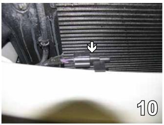
10. On the back side of the bumper, unplug the air temperature control. Remember to replug after the bumper is reinstalled.
