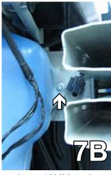
On the passenger side, using a 10MM socket, remove the three bolts holding the washer reservoir. Unplug the wires (gray arrow) and plug the water line. Set aside to be reinstalled later.
