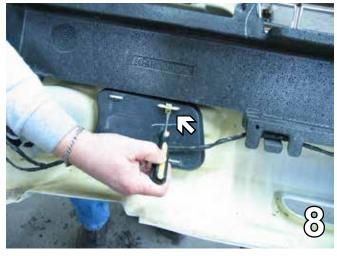
8. With the fascia upside down, push the clip down with the flat screwdriver to remove the black flat pieces. Do this on both sides of the fascia.
