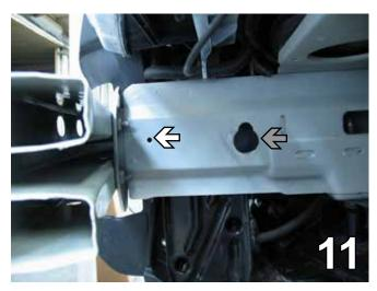
11. On the driver's side, with a 1 1/4" hole saw, drill a hole with the back existing hole to insert the wire nut for baseplate installation. Use the 13/32" drill bit to enlarge the existing hole (white arrow) as a starting point.
