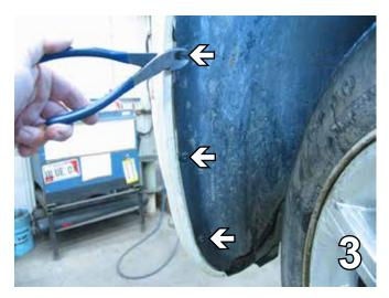
Just forward of the front tires in the wheel well, cut the three plastic push poppers with the diagonal cutters. Do this on both sides.
