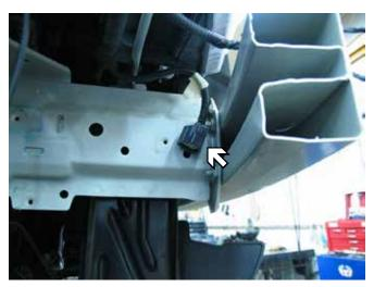
5. On the passenger behind the bumper, disconnect fascia cable from the frame. To prepare area for baseplate install.
