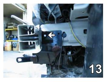
13. Slide the baseplate up from underneath, line up with the drilled hole. Make sure the baseplate is straight and clamp. Using the baseplate as a template, drill the remaining three holes with the 13/32" drill bit.
