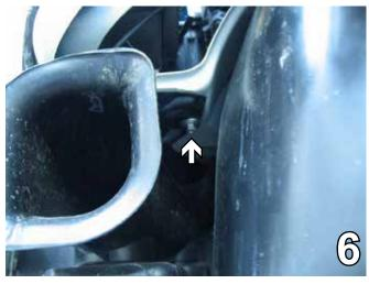
On the passenger side, use a 10MM socket to remove the bolt holding the air baffle. Set both the air baffle and the bolt aside to be reinstalled later.
