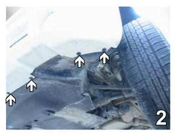
2. Remove the nine metric bolts from the lower edge of fascia all the way around with the 7MM socket. Set aside to be reinstalled later.
