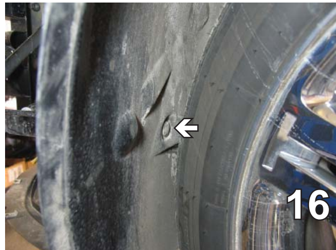
16. On the driver's side, in front of the tire, remove the push pin. Set aside to be reinstalled later.
