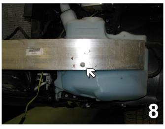
8. Using an E12 Torx, remove the inverted bolt from the front of the bumper. Set aside to be reinstalled later.
