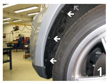
Remove three push pins just forward of the front tire on the wheel well. In the corner of the fascia using a T25 Torx, remove one screw. Do this on both sides. Set the push pins and the screw aside to be reinstalled later.
