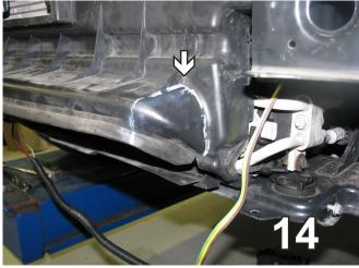
14. After the bumper has been removed using a hack saw blade trim the corner of the plastic guard. Do this on both sides.
