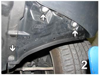
Forward of the front tire on the bottom of the fascia, remove three metric bolts. Do this on both sides. Set the bolts aside to be reinstalled later.
