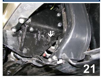
21. Apply Loctite and tighten the 3/8-16 x 1 1/2" bolts with 3/8" lock washers to the 3/8-16 nut plates. On the inside of the top two side holes insert 1/2" flat washers. Reinstall the bumper.
