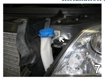
7. Using the T30 Torx, remove the bolt on the top of the washer reservoir. Set the bolt aside to be reinstalled later. On the back of the washer reservoir unplug the water lines and the electrical unit. Plug the water lines.
