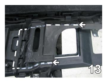
13. On the back side of the fascia, cut straight across to the inside of the slot opening. Cut only the back piece not the front fascia, Do this on both sides.
