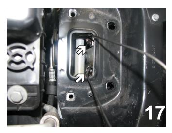
17. Insert 3/8-16 x 1 1/2" bolts with 3/8 lock washers and 3/8 nut plates inserted inside the frame rail to align with drilled holes. Do this on both sides.
