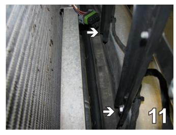
11. Using a 10MM socket, remove the two bolts from the back of both struts coming down from the hood latch. Set the bolts and the bumper aside to be reinstalled later.
