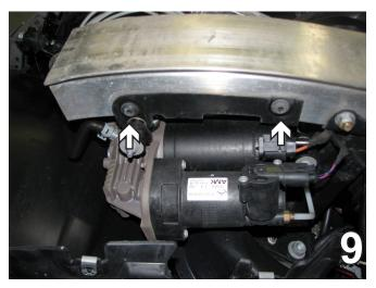
Remove the two bolts attaching the air compressor bracket on the passenger underside of the bumper using a T45 Torx. Set the bolts and bracket aside to be reinstalled later.
