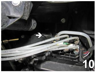
10. On the passenger side using a 13MM socket with extension, remove the nut from the air compressor. Carefully tie the compressor up out of the way and set the nut aside to be reinstalled later.
