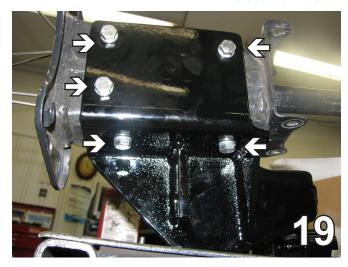
19. On the passenger side using the baseplate as a template with a 13/32" drill bit, drill the three holes on the side and two on the bottom. Insert into the holes 3/8-16 x 1 1/2" bolts with 3/8" lock washers, attach to a 3/8-16 nut plates on the inside. On the inside of the top two side holes insert 1/2" flat washers. Use Loctite on all bolts.
