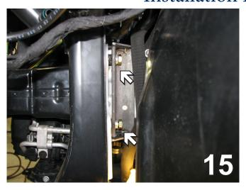
15. Using a T55 Torx, remove the two bolts behind where the washer reservoir had been. Put the bracket on with the bushings toward the front of the vehicle and line up with the holes on the back side of the frame. Insert a 10MM-1.5 x 40MM bolt with 10MM lock washer and 10MM flat washer. Do this on both sides.
