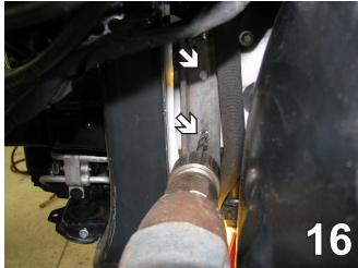
16. Using a 13/32" drill bit with the bracket as a template, drill two holes in the side of the frame rail. Do this on both sides.
