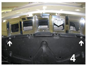
4. On the outside of the push pins, remove the two bolts. Pull the fascia forward from the corners to the front of the vehicle to unsnap. On top next to the headlights lift up over the tooth. Disconnect the fog lights on both sides. Set fascia and pins aside carefully to be reinstalled later.
