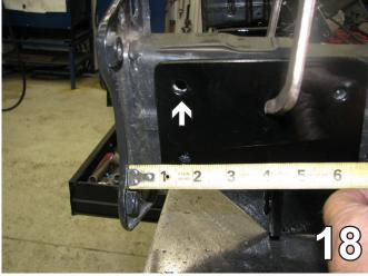
18. Set the frame extension provided aside with the base plate on the bench. Align the base plate 1" from the back of the frame rail, flush with the bottom and clamp. Do this on both sides. On the driver's side, using the base plate as a template drill the top back hole with a 13/32" drill bit and loosely bolt. Then drill the remaining two holes on the side and two on the bottom.
