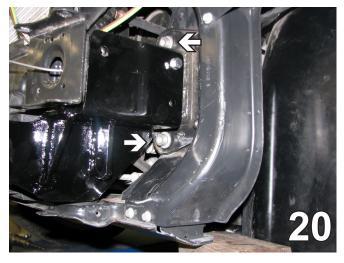
20. Cut the wire from the nut plate protruding out of the frame extension. Apply Loctite on the two T55 Torx bolts and hand tighten into the top and bottom of the frame extension to reinstall it. Do this on both sides. Realign the bumper to be sure it lines up with the two holes on the top of the frame extension on both sides. Apply Loctite to the two outside T55 bolts and tighten them first. Then tighten the two inside T55 bolts.
