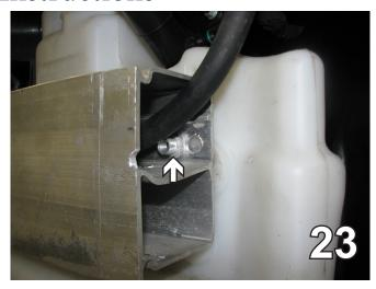
23. Slide the washer reservoir up from the bottom underneath the bumper. Using a 13/32" brill bit, drill another hole between the original and the end of the bumper. Attach with a 3/8-16 x 1" bolt and a 3/8" whiz nut. On the bottom, insert a 1/2" tube, with a 1/4" flat washer and a 6MM-1 x 30MM bolt.
