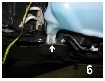
6. Using a 10mm socket, remove the bolt from the bottom of the washer reservoir. Set the bolt aside to be reinstalled later.
