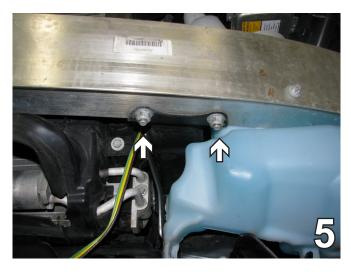
4. Using a 16mm socket, remove the two bolts underneath the bumper. Set aside to be reinstalled later.
