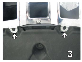
On the bottom of the fascia in the middle, remove two push pins. Set aside to be reinstalled later.
