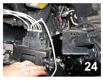
24. On the passenger side, reinstall the air compressor using the Torx bolts and the metric bolt. Reinstall the fascia, bolts and push pins.
