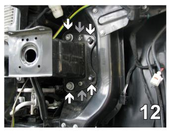
12. Using a T55 Torx remove the four bolts from the top and bottom of the frame extension (white arrows). The two on the outside must be removed from the back side. Using a 10MM socket remove the bolts in the middle, top and bottom (gray arrows). Do this on both sides. Set the bolts aside to be reinstalled later.
