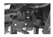
9. Bolt the baseplate to the side plates use the 1/2" hardware as shown in drawing on the last page. Tighten bolts according to the chart in the General Instruction Sheet.
