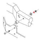
7. Remove the existing bolt from the frame and bolt the side plates with the spacers to the side of each frame using the  $1/2 \times 4$ " Hex bolt and 1/2" hardware.
