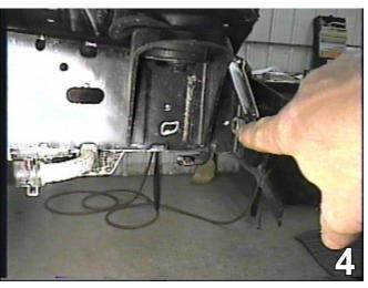
4. Remove the air dam and set aside to be reinstalled later. Using a 15MM socket remove four metric nuts from the metal bumper. Set the metric nuts aside to be reinstalled later. Using the 10MM socket, remove the air bag sensor from the cross member and set out of the way.
