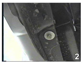
Using at 10MM socket remove two metric bolts with 10MM socket and push pins on the bottom side of fascia. There is a (the 2005 models have two) 10MM bolt to remove inside the wheel well. Do this to both sides of the vehicle. Set the metric bolts aside to be reinstalled later.
