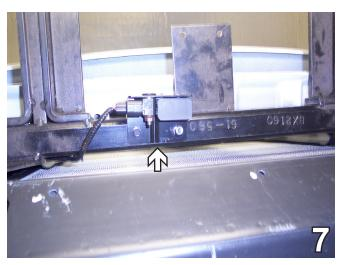
2002-03 Models: Using the air bag sensor as a template, mark and drill two holes on the bottom of the baseplate's cross tube with the 17/32" drill bit. Align the air sensor to drilled holes and install using the 1/4" self tapping screws **Do Not Over Tighten.**
