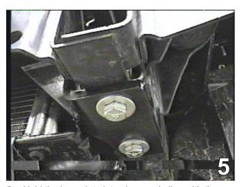
5. Hold the baseplate into place and align with the existing holes on the bottom side of the frame. Install the 1/2-13 x 1 3/4" hex washer, 1/2" lock washer, and the 1/2" flat washer. Then insert the 1/2-13 nut plate into the frame end. (See LOCTITE note)
