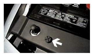
Unscrew 3 pins from black plastic on the top edge of fascia, lift up and set aside.
