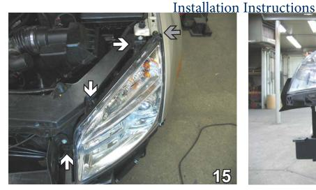
15. Using the 10mm socket, remove three metric bolts from the headlight assembly (see white arrows). Remove one pushpin from the headlight assembly's upper, outside edge (see grey arrow). Do this to both sides of the vehicle. Set bolts and pushpins aside to be reinstalled later.
