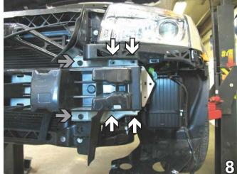
8. Using the 13mm socket, remove four metric bolts from the bumper bracket, two on the top and two on the bottom (see white arrows). Using the 10mm socket, remove two metric bolts from the side of the bumper bracket (see grey arrows). Do this to both sides of the vehicle. Pull the metal bumper forward to remove. Set bolts and metal bumper aside to be reinstalled later.
