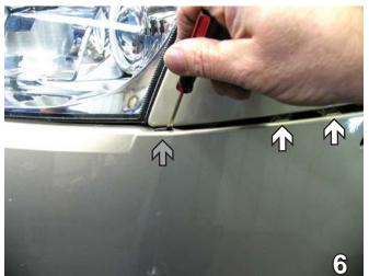
6. Release two tabs from the front fascia, between the turn signal marker and the headlight (see white arrows) and one eyelet, just behind the headlight (see grey arrow). Do this to both sides of the vehicle. Pull fascia forward to remove. Set fascia aside to be reinstalled later.
