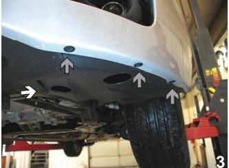
Using the 7mm socket, remove three metric bolts from the bottom edge of the fascia just forward of the front tire (see grey arrows) and one metric bolt from the back edge of the bellypan (see white arrow). Do this to both sides of the vehicle. Set bolts aside to be reinstalled later.
