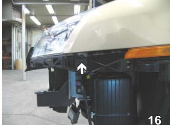
16. Using the 10mm socket, remove one metric bolt from the fender, just forward of the turn signal marker. Disconnect electrical and pull headlight forward to remove. Do this to both sides of the vehicle. Set bolts and headlight assemblies aside to be reinstalled later.
