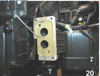
20. Remove the metal bumper. Insert the 3/8-16 nut plates into the frame rail to align with the 3/8-16 x 1 1/2" bolts and tighten with the 9/16" socket. Do this to both sides of the vehicle. Remove the vise grips.
