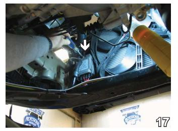
17. Using the 25 Torx socket, remove the bolt in the cut away area above the fan modulator, behind the radiator on the driver's side. Move the fan modulator out of the way to clear the area for baseplate drilling. Set bolt aside to be reinstalled later.
