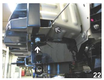
22. Using the baseplate as a template, drill into the bottom of the metal bumper using the 17/32" drill bit. Insert the 1/2-13 x 1 1/2" bolt and 1/2" lock washer (see white arrow). Insert 1/2-13 nut plate (see grey arrow) and tighten to the bolt with the 3/4" socket. Do this to both sides of the vehicle.
