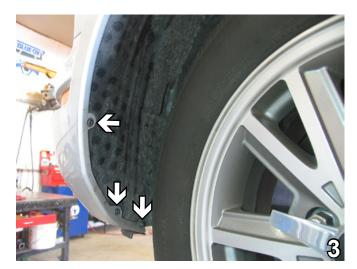
Just forward of the front tire, on edge of fascia, remove three Phillips screws. Do this to both sides of the vehicle. Set screws aside to be reinstalled later.
