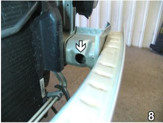
8. Using the 1 1/4" hole saw, drill a hole on the inside edge of frame rail. Do this to both sides of the vehicle. Reinstall metal bumper.
