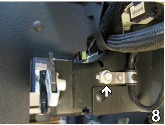
Using the 13MM socket, remove the metric bolt from the lower coolant line on the passenger's side, as indicated by the white arrow in the photo above. Some models may have a Block Heater cord bracket in this area to remove, as indicated by the grey arrow in the photo above.
