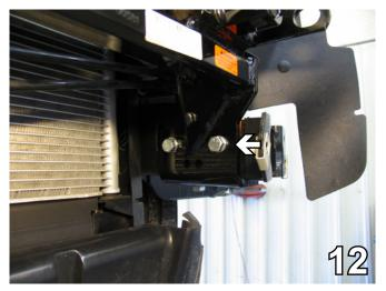
12. Insert the 1/2"-13 whiz nuts to align with the drilled holes inside the frame rail and tighten the 1/2"-13 x 1-3/4" hex bolts and 1/2" lock washers. Do this to both sides of the vehicle. Cut nut plate wires to make them flush with the end of the frame rail. This prepares the area for the metal bumper reinstallation.
