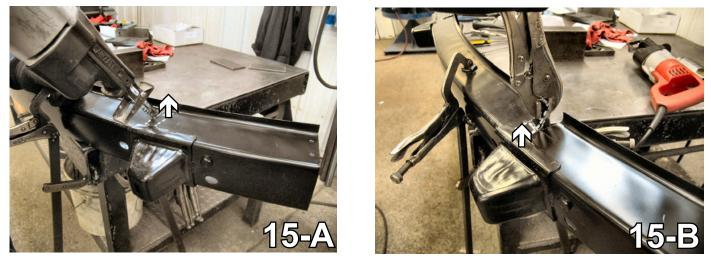
15. Secure the metal bumper to a work bench with the vise grips and cut designated areas from the previous step with the reciprocating saw. After cutting, clamp vise grip to the cut portion to be removed and move vise grip back and forth until cut portion breaks. Reinstall metal bumper to verify enough of metal bumper is removed. Trim as needed and reinstall bumper with existing hardware.
