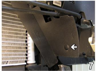
7. Remove the Christmas tree pushpin from the frame rail. Remove the air dam. Air dam will **NOT** be reinstalled. Do this to both sides of the vehicle.
