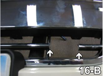
Using a utility knife, cut the fascia horizontal bar starting at the outer vertical bar and 3-1/2" out toward the edge. Do this on both sides of the fascia.
