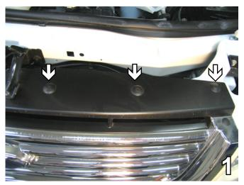
Using a Phillips screwdriver, remove three
