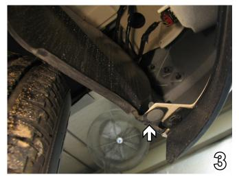
Just forward of the front tire on the fascia's lower edge, remove one (1) Christmas tree pushpin. Do this to both sides of the vehicle. Set pushpins aside to reinstall later.
