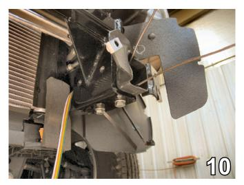
Insert the 1/2"-13 whiz nuts through the frame rail opening and align with the drilled holes. Insert the 1/2"-13 x 1-3/4" hex bolts and 1/2" lock washers and tighten. Do this to both sides of the vehicle.
