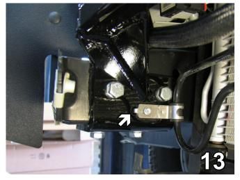
13. Insert the bent end of coolant bracket into the smaller front hole provided in baseplate on the passenger's side. Drill the self drilling screw in bracket hole provided in baseplate and into frame. BE SURE TO USE LOCTITE® RED ON ALL BOLTS BEFORE TIGHTENING. TIGHTEN ALL BOLTS ACCORDING TO THE TORQUE CHART.
