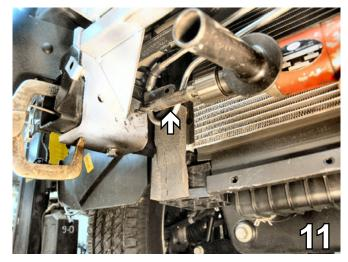
11. Using the baseplate as a template, drill the two (2) holes in the side of the frame rail with the 17/32" drill bit. Do this to both sides of the vehicle. Protect coolant pipe line when drilling (note the section of pipe on the drill bit).
