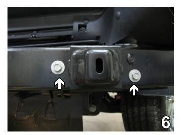
6. Using the 15MM socket, remove the two (2) metric bolts from the front of the metal bumper. Do this to both sides of the vehicle. Push down hard and out then pull the bumper forward. Set the bumper and metric bolts aside to be reinstalled later.
