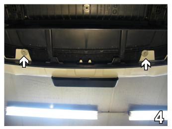
4. Using a 10MM socket, remove the two (2) metric bolts from lower tabs on the bottom edge of the fascia. Set the bolts aside to be reinstalled later.
