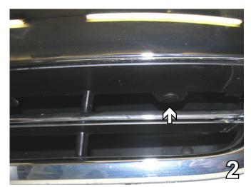
2. Remove the four (4) pushpins from upper fascia opening just behind the license plate bracket. Do this to both sides of the vehicle. Set pushpins aside to be reinstalled later.
