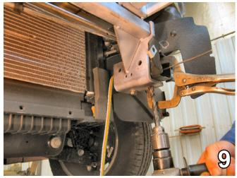
9. Slide baseplate between frame rails. Then slide baseplate forward just behind weld of the bumper bracket. Using vise grips, clamp in place to the bottom of the frame rail. Do this to both sides of the vehicle. Using the baseplate as a template, drill the two (2) bottom holes into the frame rail with the 17/32" drill bit. Do this on both sides of the vehicle.
