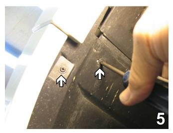
Just forward of the front tire on the fascia's corner, remove the two (2) screws with a Phillips screwdriver. Do this on both sides of the vehicle. Pull fascia corners down, then forward to release. Disconnect electrical connections. Set the fascia and screws aside to be reinstalled later.
