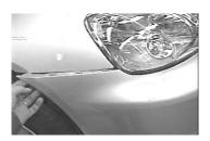
5. Pull out on the bumper fascia to release. It is snapped under the headlights also. Set fascia aside.
