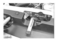
1. Open the hood and remove the push pins from the top of the bumper fascia.
