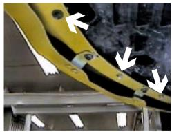
**4.** Forward of front tires on lower edge of front fascia are three metric bolts to remove with the 10MM socket, both sides.
