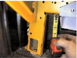
7. Using the tape measure, mark 2 1/2" down from the bottom of frame on air dam (view of passenger's side).
