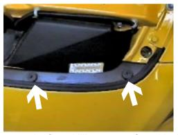
Remove the five phillips screws from black plastic cover on top side of fascia with the phillips screw driver, lift cover and set aside.
