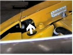
2. Remove the black metric bolt from inside fender from opening at the ends of black plastic with the 10MM socket, both sides.
