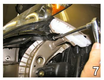
7. Using the 10MM socket, remove one metric bolt from the side of the headlight assembly. Do this to both sides of the vehicle. Set the bolts aside to be reinstalled later.
