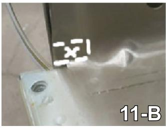
11. Cut the front webbing on the top edge of the frame and the 1/2" above the frame with the reciprocating saw. Bend the webbing toward the headlight area. Do this to both sides of the vehicle. This will open the area for the baseplate installation.
