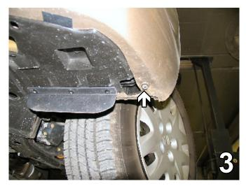
Using a 10MM socket remove one metric bolt from just forward of the front tire. Do this to both sides of the vehicle.
