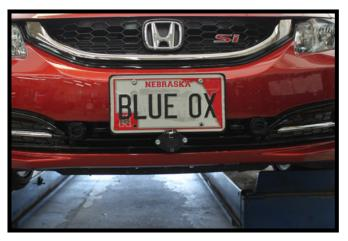
18. Hold the fascia as close to its original position, mark and trim the fascia around the convenience links and attachment tabs. Reinstall the fascia.
