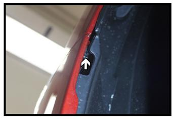
Using a Phillips screwdriver, remove the screw from the wheel well where the fascia meets the fender. Do this on both sides of the vehicle.
