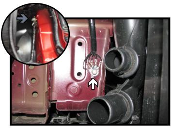
10. On the driver side, using a 10MM socket, remove the ground wire (white) and relocate it to the upper ground wire location behind the headlight, reusing the bolt from the lower location (inset).
