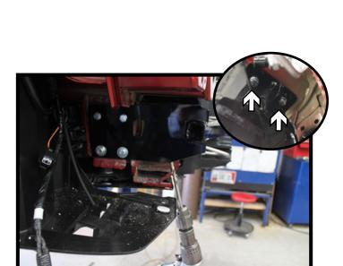
15. Using a 13/32" drill bit, drill the bottom holes thru the frame. Install 3/8"-16 x 1-1/2" bolts with 3/8" lock washers into the holes with 3/8"-16 nut plates in the frame. Do this on both sides of the vehicle. Fully tighten all hardware.
