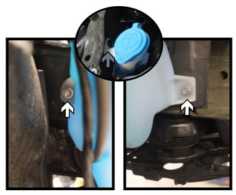
Using a 10MM socket, remove the two (2) screws from washer reservoir (white). Remove the push pin from the filler neck next to the cap (gray). Disconnect all lines from the reservoir and set aside.
