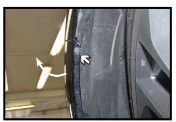
Using a Phillips screwdriver, remove the screw from the wheel well. Do this on both sides of the vehicle.
