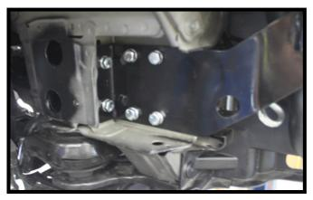
Continue to drill the remaining holes thru the frame. Install 3/8"-16 x 1-1/2" bolts with a 3/8" lock washers into the holes and secure with a 3/8" nut plates on the inside of the frame. Do this on both sides of the vehicle. Fully tighten all fasteners.
