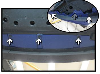
4. On the underside of the fascia, remove the seven (7) push pins (white). There are three (3) in the middle and four (4) along the outer edges. Using a Phillips screwdriver, remove the two (2) screws (gray).
