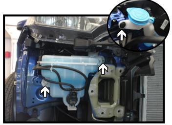
8. On the passenger side, remove the push pin from the washer reservoir neck (inset). Using a 10MM socket, remove the two (2) screws from the reservoir. Disconnect/plug all lines and set the reservoir aside.
