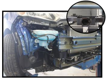
12. Reinstall the bumper and washer reservoir. Attach the temperature sensor to the baseplate as shown with the supplied zip ties (inset).
