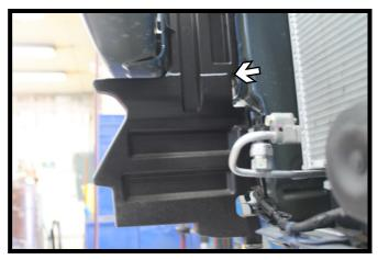
5. Trim off the plastic shrouding flush with the bottom side of the bumper. Do this on both sides of the vehicle.
