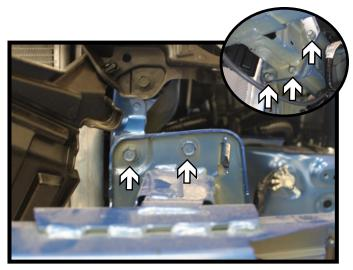
Using a 12MM socket, remove the five (5) bolts on both sides of the bumper and set it aside.
