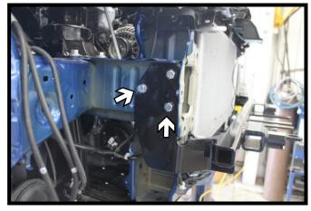
10. Using a 3/8" drill bit, drill the remaining holes thru the frame. Install a 3/8"-16 x 1-1/4" bolt into the lower front hole with a 3/8" lock washer and nut on the inside of the frame. Then a 3/8"-16 x 1-1/4" bolt with 3/8" lock washer into the back hole with a 3/8" nut plate on the inside of the frame. Do this on both sides of the vehicle. Fully tighten all hardware.
