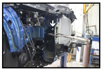
9. Position the baseplate onto the frame so it is touching the top and front frame lips. Level and securely clamp the baseplate. Using a 3/8" drill bit, drill the top front hole thru the frame. Install a 3/8"-16 x 1-1/4" bolt into the hole with a 3/8" lock washer and nut on the inside of the frame. Do this on both sides of the vehicle. Fully tighten all hardware.
