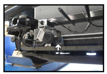
13. **Optional Breakaway:** Using a 12MM socket, remove the existing screw and reinstall with the breakaway bracket. Install the breakaway switch to the bracket with the supplied 1/4" hardware.
