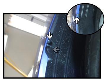
3. In the wheel well, remove the push pin just below the fascia joint (gray). Using a Phillips screwdriver, remove the two (2) screws (white). There is one (1) at the fascia joint and one (1) along the outer edge below the joint. Do this on both sides of the vehicle.
