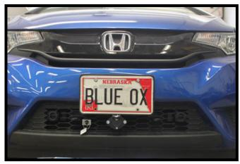
14. Hold the fascia as close to its original position, mark and trim the fascia around the convenience links and attachment tabs. Reinstall the fascia and fascia cover.
