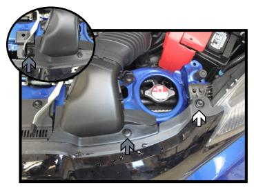
2. On the driver side, remove the push pin from outer edge (white). Then remove the two (2) expansion rivets on either side of the air intake tube (gray) by depressing the center of the rivet.
