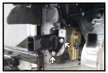
14. Install the baseplate into the frame. Start the rear 3/4" hardware into the rear hole but do not fully tighten (gray). Install the 8MM hardware into the front holes and fully tighten. Once the front bolts are tightened, fully tighten the rear 3/4" bolts.
