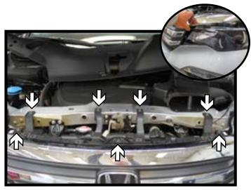
Using a 10MM socket, remove the seven (7) screws from the top edge of the fascia.
