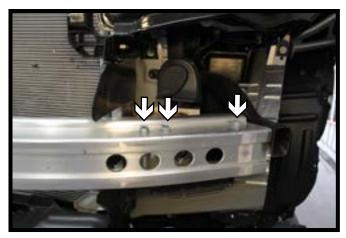
6. Using a 14MM socket, remove the six (6) bolts from the bumper. There are three (3) on each side. Set the bumper aside it will not be reinstalled.
