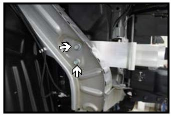
7. Using a 14MM socket, remove the two (2) bolts from the frame braces. Do this on both sides of the vehicle. The braces will not be reinstalled.
