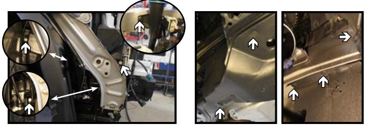
10. Using a 10MM socket, remove the three (3) screws from the washer reservoir. Then remove the one (1) push pin from the filler neck (left).
