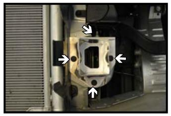
Using a 12MM socket, remove the three (3) bolts from the face of the frame extension. Do this on both sides of the vehicle.
