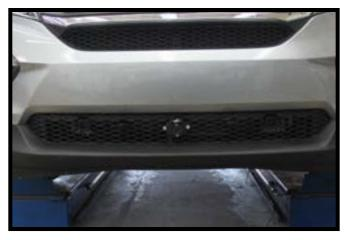
16. Hold the fascia as close to its original position, mark and trim the fascia around the convenience links and attachment tabs. Reinstall the washer reservoir, air baffle, fascia and fascia cover.
