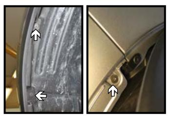
4. Using a phillips screwdriver, remove the three (3) screws from the edge of the wheel well (left). The upper two screws are shown the third screw is below.
