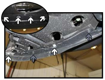
Using a 10MM socket, remove the eight (8) screws from the underside of the fascia. There are two (2) in each corner and four (4) in the middle (white).
