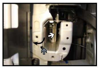
12. On the front part of the frame pocket, bend the tab forward so it is flush or just past the inside face of the frame (gray). Inside the frame pocket, bend the inner structure in so that the 3/4" nut will clear. Do this on both sides of the vehicle.
