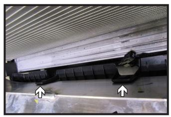
9. Remove the two (2) push pins attaching the plastic shroud to the back side of the bumper.
