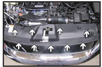
Remove the nine (9) push pins from the fascia cover. There are five (5) on driver side and four (4) on the passenger side. Set the cover aside.
