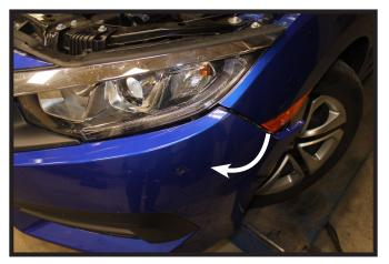
Pull the corners of the fascia away from the vehicle disconnecting any electrical connections and set the fascia aside.
