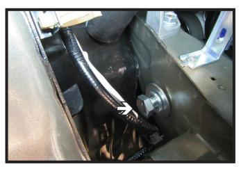
17. Start the 5/8" bolt with flat washer and lock washer. Do not tighten fully. Do this on both sides of the baseplate
