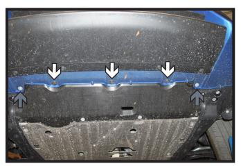
Using a 10MM socket, remove the bolt (gray) from the underside of the fascia. Then remove the two (2) push pins (left photo). Do this on both sides of the vehicle. Using a T30 Torx, remove the two (2) bolts towards the center (gray). Then remove the three (3) push pins (right photo).
