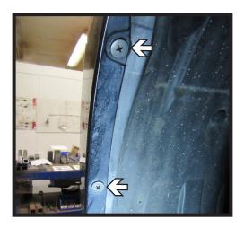
Using a Phillips screwdriver, remove the two (2) screws from the edge of the wheel well. Do this on both sides of the vehicle.
