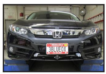
22. Hold the fascia as close to its original position, mark and trim the fascia around the convenience links and attachment tabs. Reinstall the headlights, fascia and fascia cover.
