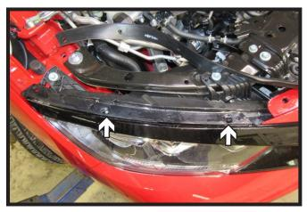
5. **2019 Models:** Remove the plastic piece above the head light using Phillips screw driver to press down on two (2) snaps. Do this on both sides of the vehicle.
