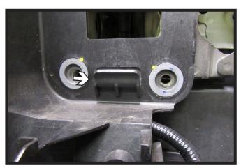
12. Using a reciprocating saw, trim the hook at the lower bumper bolt location flush with the frame. Do this on both sides of the vehicle.
