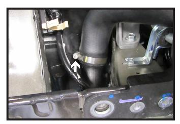
Using a 10MM socket remove the bolt attaching the clamp to the turbo air coolant tube.
