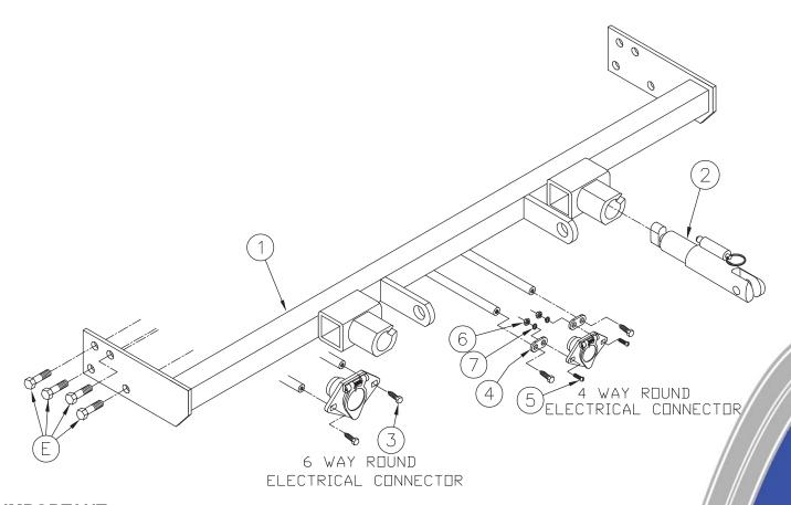
**IMPORTANT:** Use only genuine factory replacement parts on your Base Plate. Do not substitute homemade or nontypical parts. If a bolt is lost or in need of replacement, for your safety and the preservation of your Base Plate, be sure to use a replacement bolt of the same grade (Usually Grade 5, refer to parts list). Repair parts may be ordered through your nearest **Blue Ox** dealer or distributor.
