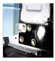
**11.** Bolt the baseplate to the frame with the six existing 10 mm bolts, and two 6mm bolts.
