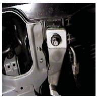
3. Remove two 6mm screws, one by each headlight.
