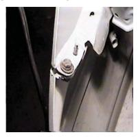
**4.** Remove the third 6mm screw on the passenger's side of facia.
