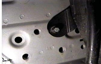
**8.** Remove the tow hooks with a 17mm socket. Remove the smaller bolt with a 10mm socket on the driver's side.
