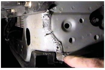
**9.** Cut the rib 4 times with a hacksaw and then bend over with a pliers as shown above.
