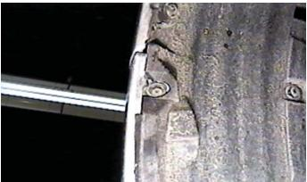
**7.** Remove the screws in the wheel well with a 8mm socket, one on each side, to remove the bumper.
