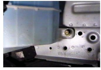
10. On the passenger's side, do the same thing, remove the bolt fastening the washer fluid container with a 10mm socket and cut the rib and bend over as in step 9.
