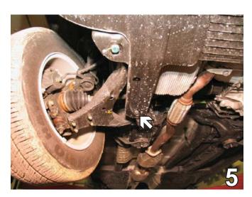
Passenger's side of the belly pan will have an additional metric bolt further back of the push pin that needs to be removed with the 12MM socket, and set belly pan aside.
