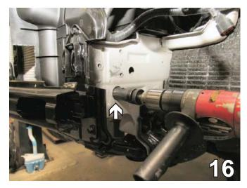
16. Using the 1 1/4" hole saw, cut an opening in the lower portion of the frame rail to use for wire nut installation, both sides as shown in photo.
