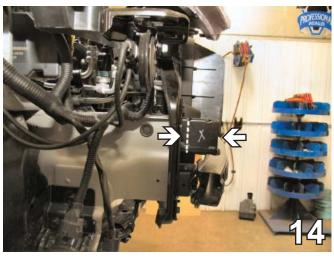
14. Measure and mark from the end of the frame extension 2 1/2" back with a marker. Remove this section from the frame extension with the reciprocating saw, both sides. Passenger's side is shown.
