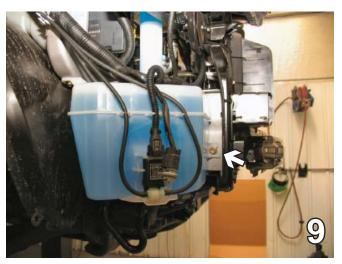
Remove front metric bolt from the washer reservoir on the passenger's side using the 10MM socket.
