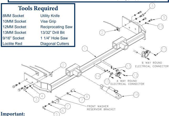
Use only genuine factory replacement parts on your baseplate. Do NOT substitute homemade or non-typical parts. If a bolt is lost or in need of replacement, for your safety and the preservation of your baseplate, be sure to use a replacement bolt of the same grade. In most cases it will be Grade 5-please reference the parts list above. Replacement parts may be ordered through your nearest Blue Ox\* dealer or distributor, or call our Customer Care Team at (402)385-3051 or toll free (888) 425-5382.
