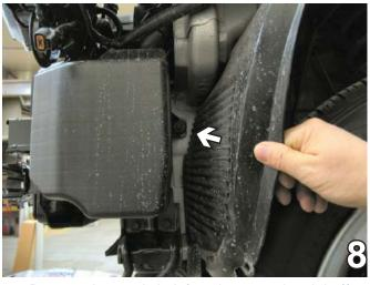
Remove the metric bolt from between the air baffle and wheel well using the 12MM socket, pull the air baffle down to disconnect from upper tube and set aside.
