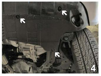
Remove the two metric bolts from the belly pan just inboard of the tie down brackets with the 12MM socket, both sides. Remove the Phillips head push pin, both sides (driver's side is shown).
