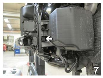
7. Using the 12MM socket, remove the two front metric bolts from the air baffle on the driver's side.
