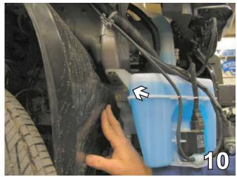
Separate the wheel well from the back side of the reservoir and remove the two metric bolts using the 10MM socket, pull reservoir down, unplug electrical connections, disconnect and plug water lines, set aside.
