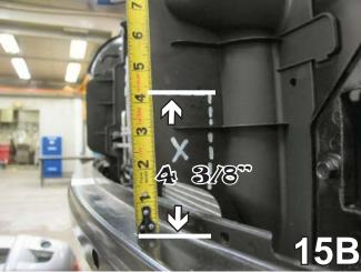
15. Measure and mark 2 1/4" horizontally from the front edge of air dam to the radiator and vertically 4 3/8" from the top of metal bumper to the air dam. Remove this portion of the air dam with the utility knife, both sides.
