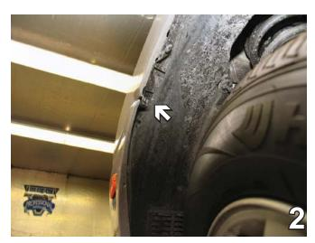
2. Remove the metric bolt on the upper corner of fascia just forward of front tire with the 8MM socket, both sides.
