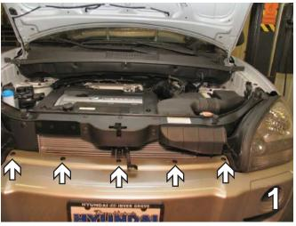
1. Remove the five push pins from the top edge of fascia between head lights.
