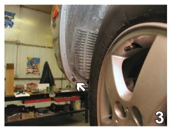
Remove the Phillips head push pin from lower corner of fascia just forward of front tire with the Phillips screw driver, both sides.
