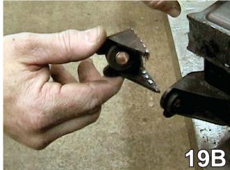
19. Using the utility knife, cut and remove the front upper bolt bracket from the air baffle flush with the main body. Reinstall air baffle on driver's side.
