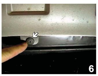
6. Remove Phillips head push pin on the lower edge of fascia, pull fascia forward, unplug all electrical connections and set fascia aside.
