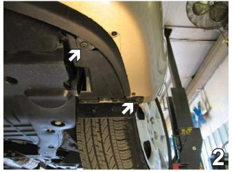
Remove two Phillips push pins on the underneath corner of fascia, just forward of the wheel well.
