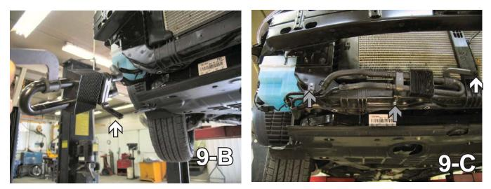
9. Using the 10MM socket, remove three bolts from coolant tubing (see 9-A). Relocate driver's side bolt to lower existing threaded hole in coolant tubing bracket. Bend middle coolant tube bracket 90 degrees toward the radiator (see 9-B). Refasten using two self drilling screws (gray arrows). Photo 9-C shows relocated coolant tubing.
