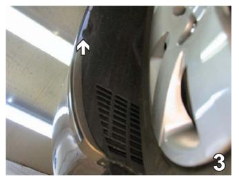
3. Using a 10MM socket, remove one bolt from the front fascia, inside the wheel well. Do this to both sides of the vehicle. Set bolts aside to be reinstalled later.
