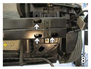
8. Using the 12MM socket, remove three bolts from the metal bumper and set aside to be reinstalled later. Do this to both sides of the vehicle. Release clips and remove air dam from the side of the radiator. Do this to both sides of the vehicle.
