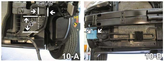
10. Using a reciprocating saw, trim horizontally 2 1/2" just behind the bumper bracket from the outside edge of the radiator support into the frame rail edge. Trim vertically 4" from the bottom, of the radiator support to the horizontal to open area for baseplate installation. Do this to both sides of the vehicle.
