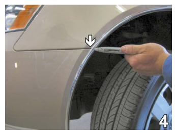
4. If necessary, use a utility knife to cut the wheel well trim so the fascia may be removed. Pull the front fascia forward and set it aside carefully.
