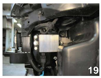
19. Reinstall the fan controller to its original position using the 6MM-1.00 x 45MM hex bolt, 6MM lock washer and four 1/4" flat washers.
