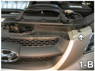
1. Remove seven Phillips screws from the top edge of the front fascia, as indicated by the white arrows in photo 1-A. Remove two bolts from the top side of the fascia using a 10MM socket, as indicated by the arrow in photo 1-B. Set push pins and bolts aside to be reinstalled later.
