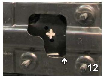
Using a 1 1/4" hole saw drill a 1 1/4" hole in the center of the metal bumper bracket opening. (It may be necessary to bend the bumper bracket to gain access.) Do this to both sides of the vehicle.
