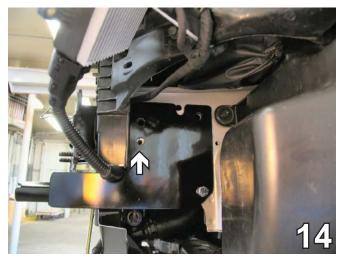
14. Using large vice grips, clamp the baseplate in place by aligning the front, center hole with the existing front hole for the fan controller on the driver's side (see white arrow in photo above). Insure the baseplate is level before clamping on the passenger's side.
