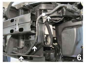
6. Remove three clips from electrical cable. Move the cable aside to clear area for baseplate installation.
