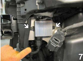
7. On the driver's side, just behind the metal bumper, remove two bolts with the 10MM socket and set the fan controller and bolts aside to be reinstalled later.
