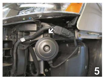
Using a 10MM socket, remove one bolt from the horn bracket, as indicated by the white arrow.
