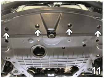
11. Using a 10MM socket, remove four bolts underneath the belly pan. Pull the belly pan forward and set aside to be reinstalled later.
