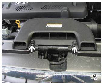
2. Using a 10MM socket, remove two metric bolts from the air intake housing. Set bolts aside to be reinstalled later.
