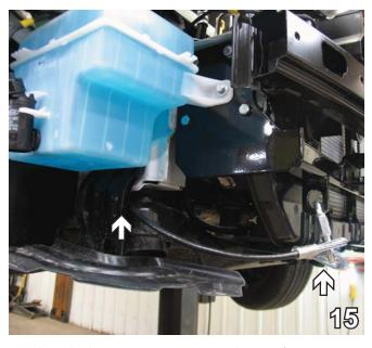
15. Attach the permanent baseplate safety cables to the provided convenience link on the baseplate. The photo above shows the recommended installation of the cables to frame of vehicle. Additional options may interfere with suggested mounting; in this case secure the cables to a solid piece of the frame as described in the instructions included with the permanent baseplate safety cables. Be sure the safety cables do not rub against any hoses or moving parts. Do this to both sides of the vehicle.
