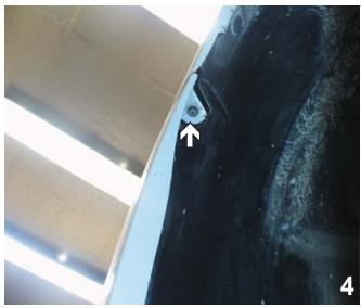
Using a Phillips screwdriver, remove one plastic Phillips pushpin just forward of the front tire, on the wheel well. Do this to both sides of the vehicle. Set pushpin aside to be reinstalled later.
