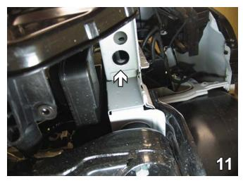
11. Using a 1 1/4" hole saw, drill a hole in the bottom of the frame for the nut plates. Do this to both sides of the vehicle.
