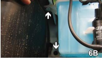
Remove water reservoir from passenger side, by using a 10MM socket to remove two metric bolts and by loosening up a Phillips screw. Set water reservoir and bolts aside to be reinstalled later.
