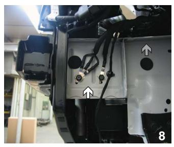
8. You will need to relocate the ground wires located on the drivers side (see white arrows), to the area indicated by the grey arrow.
