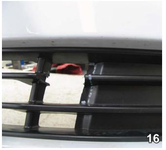
16. Align the fascia to its original position, and using a hack saw blade, remove bar piece from grille as shown in photo above. You will also need to remove area outlined with white dashed lines. This is going to allow for attachment tab receiver to come through. Do this to both sides of the vehicle.
