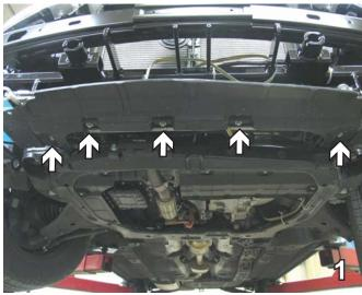
Using a 10MM socket, remove five metric bolts from the belly pan. Set belly pan and bolts aside to be reinstalled later.
