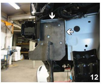
12. Slide baseplate up so it measures 3/16" down from top of frame and the back of the baseplate is straight with the frame. Clamp the baseplate into place with vise grips. Do this to both sides of the vehicle.
