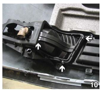
10. Using a reciprocating saw, remove plastic area (see white arrows) located on the back of the fascia behind the running lights. Do this to both sides of the fascia.
