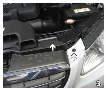
Using a Phillips screwdriver, remove two
