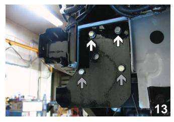
13. Using the baseplate as a template, drill the two bottom and top holes. Insert the nut plates into the bottom of the frame and align with top drilled holes. Insert a 3/8-16x1 1/4" hex bolt and 3/8 lock washer into the top two holes and tighten down (see white arrows). Insert a 3/8-16x1" hex bolt into the bottom two holes and tighten down with a 3/8-16 hex nylon lock nut (see grey arrows). Do this to both sides of the vehicle.
