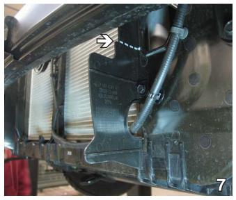
7. Using a utility knife, remove plastic guard by cutting along white dashed line indicated in photo above. Do this to both sides of the vehicle.
