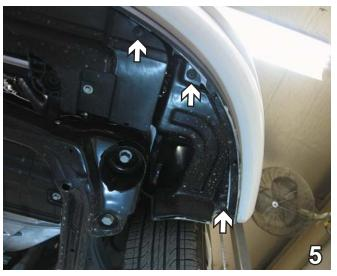
5. Using a Phillips screwdriver, remove three plastic Phillips pushpins from just forward of the front tire along the bottom edge of fascia. The fascia is then ready to be removed from the vehicle by pulling fascia ends out to the side to release and then pulling it forward. Do this to both sides of the vehicle. Set fascia and pushpins aside carefully to be reinstalled later.
