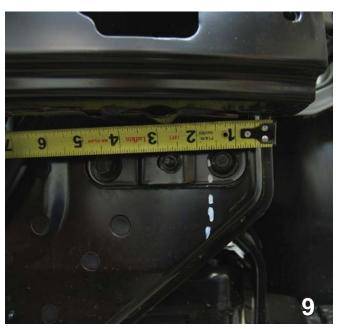
9. Using a reciprocating saw, trim out area below bumper according to the photo above. You will need to measure in 1 3/4" from the side of frame and just below metal bumper. Remove this area from both sides.
