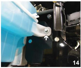
14. Reinstall the water reservoir, by inserting a 6MM-1.0x30MM hex bolt, 1/4" lock washer and 1/4" flat washer into the existing hole shown on baseplate. Use existing bolt removed in Step 6, to tighten down opposite side.
