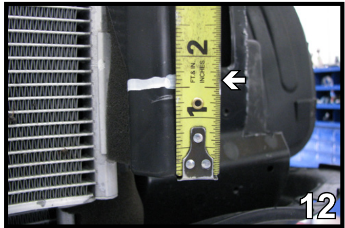
12. Mark 1 3/4" up on the plastic. Remove the piece by pulling out on the backside and lifting up. Cut the marked area. Do this on both sides.
