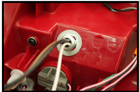
2. Drill a 1" hole to install the 3 wire automotive socket.
