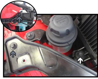
6. Underneath the passenger side headlight, using a 10MM socket, remove the screw from the brace (white). Then using a 12MM socket, remove the screws from the top and side of the brace (gray).
