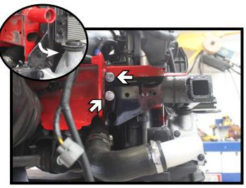
10. On the passenger side, bend the frame face over to allow nut plate access (inset). Position the baseplate onto the vehicle. Install two (2) 10MM-1.25 bolts with 10MM lock washers into the existing holes at the rear of the baseplate. Do this on both sides of the vehicle. Fully tighten all hardware.
