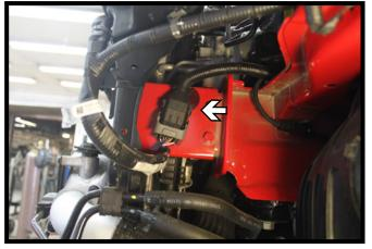
On the driver side, remove the wiring harness from the frame.
