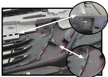
16. On the backside of the fascia, trim the tab off the edge of the grille for baseplate clearance. Also trim the tab off the upper styrofoam support. Do this on both sides of the fascia,
