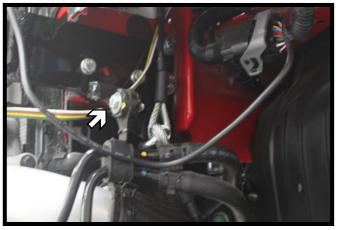
12. On the driver side, reinstall the coolant line to the baseplate tab with the existing hardware.
