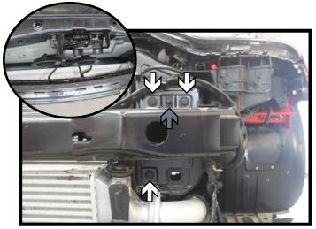
4. Unsnap the wiring loom from the backside of the fascia (inset). Using a 12MM socket, remove the three (3) bolts from the bumper (white). Then using a 10MM socket, remove the remaining bolt from the bumper (gray). Do this on both sides of the vehicle. The bumper will not be reinstalled.
