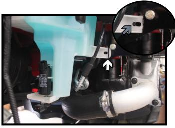
13. Trim approximately 1/4" of the tab of the washer reservoir for clearance of the bolt. Reinstall the reservoir starting the back bolt first then the front bolt. Note: The front slot may need to be elongated slightly for bolt clearance (gray).
