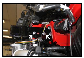
11. Using a 13/32" drill bit, drill the two (2) remaining holes in the sideplate thru the frame. Install 3/8"-13 x 1-1/4" bolts with 3/8" lock washers into the holes and 3/8" nut plates on the inside of the frame. Do this on both sides of the vehicle. Fully tighten all hardware.
