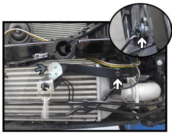
15. Optional Breakaway: Install the bracket to the existing bolt location just to the side of the intercooler (white) with three (3) flat washers behind as a spacer (inset).
