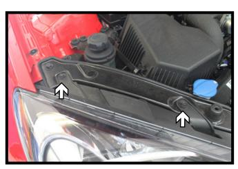
5. Using a 10MM socket, remove the two (2) screws from the passenger side headlight. Disconnect the wiring and set aside.
