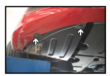
Remove the four (4) Phillips head push pins from the underside of the fascia.
