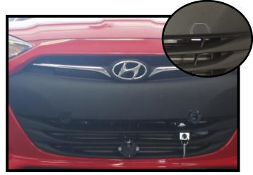
17. Hold the fascia as close to its original position, mark and trim the fascia around the attachment tabs. Reinstall the fascia.
