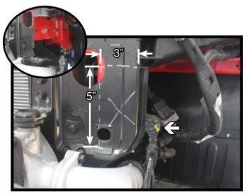
9. Using a 10MM socket, remove the screw from the cooler line. Trim the face of the frame 3" over and 5" down as shown for baseplate clearance. Do this on both sides of the vehicle.
