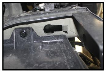
12. Using a reciprocating saw, cut two (2) slits on the bottom hole in the frame and bend the tab out to allow nut plate access. Do this on both sides of the vehicle.
