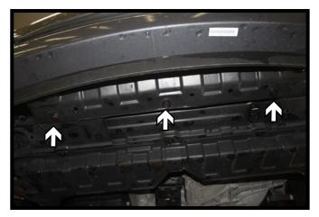
4. Using a 10MM socket, remove the three (3) screws from the middle of the fascia.
