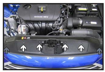
Remove the four (4) push pins from the top of the fascia cover (white). Using a 10MM socket, remove the two (2) bolts from the fascia cover (gray).
