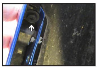
4. Using a 10MM socket, remove the one (1) bolt from the upper part of the wheel well. Do this for both sides of the vehicle.
