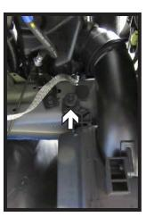
8. Remove the wire looms secured to the air baffle on the driver's side. Using a 10MM socket, remove three (3) bolts holding the baffle in place. There is one (1) on both sides of the baffle, with one (1) behind the baffle.
