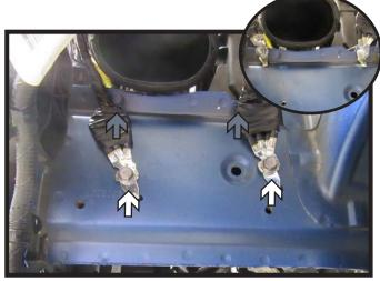
11. Using a 10MM socket, remove the two (2) bolts on the driver's side bumper horn (white). Using a 1/4" drill bit, bore the upper existing two (2) holes out (gray). Bolt the connections into these holes, as pictured above.
