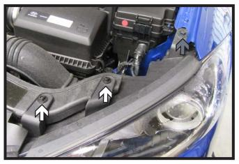
Using a 10MM socket, remove the two (2) bolts from above the headlights (white).
