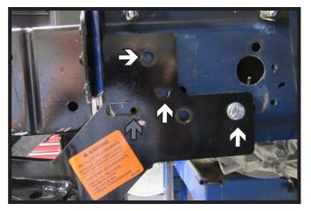
16. Install the baseplate to the frame, aligning the existing holes in the frame to the baseplate. Level and clamp in place. (It is recommended to use the existing bolts to pin the baseplate in place while leveling and clamping, then remove after baseplate bolts are installed)
