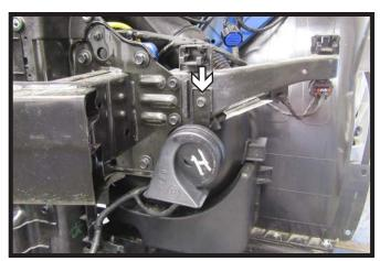
6. Using a 10MM socket, remove the one (1) bolt that secures the horn in place. Do this for both sides of the vehicle.
