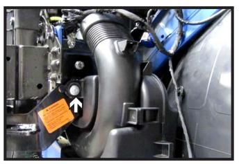
17. When reinstalling the air baffle, use the supplied 3/8" hardware to secure it through the baseplate hole.
