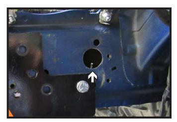
13. On each side of the frame right above the baseplate drill an 1-1/4" hole using a hole saw to use as an the access hole for the nut plates with 14" wire.
