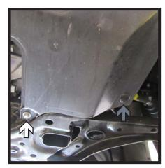
7. Using a 10MM socket, remove the four (4) bolts at the front of the belly pan. There are two (2) on each side of the vehicle (left). Next, remove the two (2) bolts (center white) and the one (1) push pin (center gray) from the back-passenger side of the belly pan. Then, remove the one (1) bolt (right white) and the one (1) push pin (right gray) from the back-driver side of the belly pan. Remove the belly pan and set aside.
