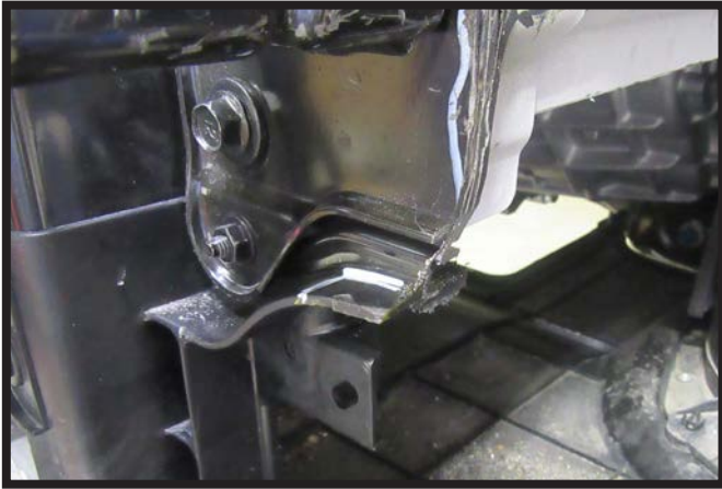
14. Using a utility knife trim the plastic piece as indicated. Do this on both sides of the vehicle.
