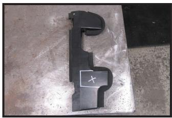
16. Slide the air baffle into place and mark the area that needs to be trimmed. Trim area and reinstall. Do this on both sides of the vehicle.
