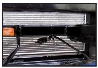
22. Using the provided zip tie, attach the temperature sensor to the baseplate as shown.
