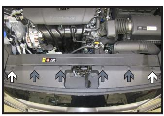
1. Using a 10MM socket, remove the two (2) bolts (white) and four (4) push pins (gray) from the top of the fascia.
