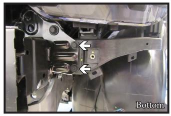
13. Using a 10MM socket, remove the four (4) bolts (white), two (2) on top and two (2) on the bottom, from the head light. Then using a 12MM socket, remove the one (1) bolt (gray) from the top corner of the head light. Remove head light and set aside to be reinstalled later. Do this on both sides of the vehicle.
