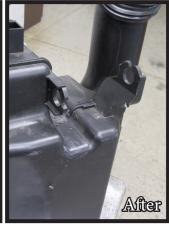
18. Remove the two (2) rubber grommets from the air baffle as shown before reinstalling.
