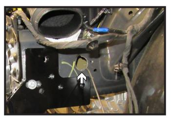
15. Using a 1-1/4" hole saw, drill out the existing hole on the side of the frame to create and access hole. Do this on both sides of the vehicle.
