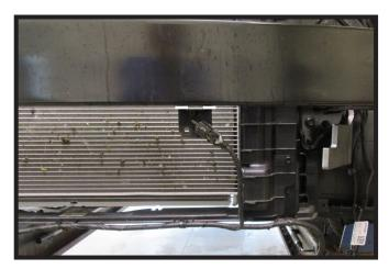
14. Using a reciprocating saw, remove the temperature sensor bracket from the bottom of the bumper. Unclip the sensor from the bracket and set aside to be repositioned later.
