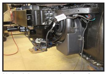
21. Attach the permanent baseplate safety cables to the provided convenience link on the baseplate. The photo above shows the recommended installation of the cables to frame of vehicle. Additional options may interfere with suggested mounting; in this case, secure the cables to a solid piece of the frame as described in the General Information sheet. Be sure the safety cables do not rub against any hoses or moving parts. Do this on **BOTH** sides of the vehicle.
