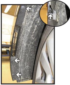
2. Remove the three (3) push pins from along the edge of the wheel well. Then using a 10MM socket remove the one (1) bolt (inset). Do this on both sides of the vehicle.
