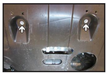
4. Using a 10MM socket, remove the four (4) bolts, two (2) on each side from the front portion of the belly pan.
