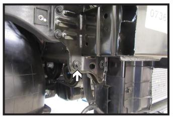
11. Using a 12MM socket, remove the one (1) bolt as shown from the bumper. Do this on both sides of the vehicle.
