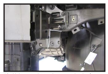
12. Using a reciprocating saw, trim the frame as indicated on both sides of the vehicle.
