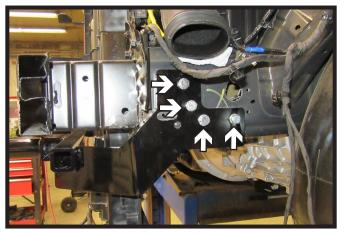
17. Using a 3/8" drill bit, drill out the four (4) holes on the side of the frame using the baseplate as a guide. Install the four (4) 3/8" bolts with hardware. Remove the 6MM bolt from the existing hole. Do this on both sides of the frame.
