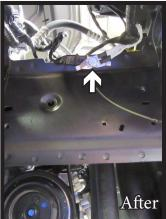
9. Using a 10MM socket, remove the two (2) bolts attaching the wires to the side of the frame. Using a 1/4" drill bit, drill a hole higher on the frame. Combine wires and reattach to the frame using an existing 1/4" bolt.
