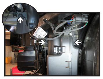
6. Using a 10MM socket, remove the three (3) bolts from the air baffle on the driver side of the vehicle. There are two (2) on the outside of the frame and one (1) on the backside. Remove baffle and set aside to be reinstalled later.
