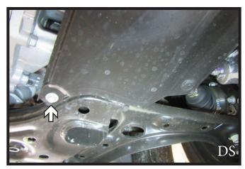
5. Using a 10MM socket, remove the two (2) bolts from the passenger side and one (1) bolt from the driver side of the belly pan. Remove belly pan and set aside to be reinstalled later.
