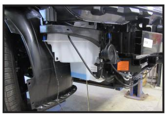
20. Reinstall the windshield washer fluid reservoir using existing hardware for back hole and provided 6MM bolt and hardware for front hole. Then reinstall horn bracket to the passenger side of the vehicle and both head lights.
