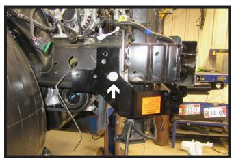
16. Slide the baseplate into place, ensure it is level, then start the one (1) 6MM bolt with hardware in the existing hole. Do this on both sides of the vehicle.
