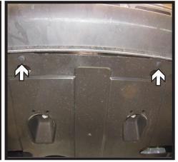
3. Remove the twelve (12) push pins from the underside of the fascia. There are two (2) next to the tire on each side (left), three (3) each side (middle), and two (2) in the center (right). Remove fascia and set aside to be reinstalled later.
