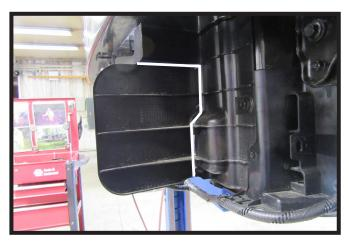
10. Using a utility knife, trim the plastic shielding on both sides of the vehicle as shown.
