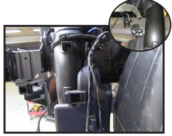
19. Reinstall the air baffle on the driver side of the vehicle using the provided 6MM bolt with hardware on the outside of the frame. Use the existing bolt and hardware on the backside of the frame (inset).
