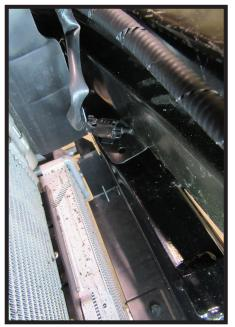
19. Reattach the temperature sensor to the bracket and the wire loom to the back of the bumper.
