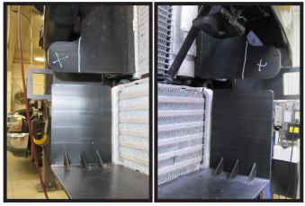
6. Trim the plastic shield as shown on both sides of the vehicle.
