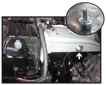
17. Install one (1) 1/2" bolt with lock washer and flat washers into the bottom of the frame, securing frame bracket. Tighten both bottom bolts at this time. Do this on both sides of the vehicle.
