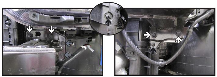
5. Using a 12MM socket, remove the four (4) bolts (white) from the bumper, two (2) on top and two (2) on bottom. Then using a 10MM socket, remove the (2) bolts (gray) from the side of the bumper and the two (2) nuts (black) from the top and bottom of the bumper. Remove bumper and set aside to be reinstalled later.
