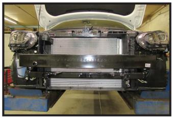
Finish reinstalling the bumper using the existing nuts and bolts.
