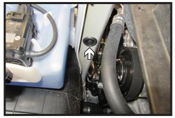
8. Remove the plastic plug on the underside of the frame. Do this on both sides of the vehicle. The plug will not be reinstalled.
