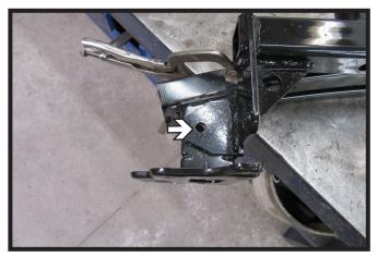
14. Using a 1/2" drill bit, drill a hole in the bottom of the bumper using the baseplate as a template. Do this on both sides of the vehicle.
