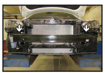
Start to reinstall the bumper by installing one (1) existing bolt at the top on each side of the vehicle.
