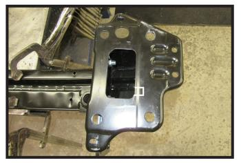
10. Using a reciprocating saw, notch and remove the indicated 1/2" x 1/2" section of the bumper to allow clearance for the frame bracket. Do this on both sides of the bumper.
