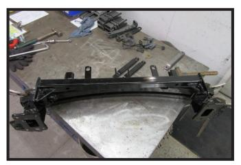
11. Set the bumper upside down on a firm level service. Place baseplate on the bumper, lining up existing holes. Clamp baseplate into place.
