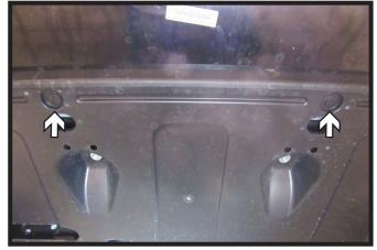
3. Remove the ten (10) push pins from the underside of the fascia, there are four (4) in each corner and two (2) in the middle.
