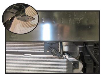
4. Unclip the temperature sensor from the bracket on the bumper and unsnap the wire loom from the backside of the bumper. Bend the temperature sensor bracket back toward the radiator as shown to allow clearance for the baseplate (inset). The temperature sensor will be reattached later.
