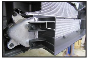
7. Trim the turbo shroud as indicated. Do this on both sides of the vehicle.
