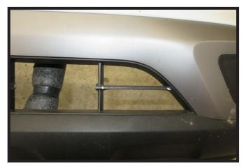
15. Remove the two (2) horizontal slats as shown on the driver side of the fascia to allow room for the removable tab, convenience link and electrical.
