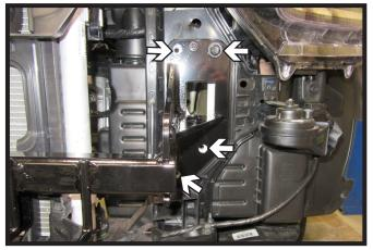
9. Lift baseplate to center rest of the holes. Reinstall the four (4) existing 10MM bolts on each side of the vehicle.
