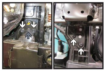
Using a 12MM socket, remove the four (4) bolts (white) from the bumper. Using a 10MM socket, remove the one (1) nut (gray) on the top of the bumper. Do this on both sides of the vehicle. Remove bumper, it will not be reinstalled later.
