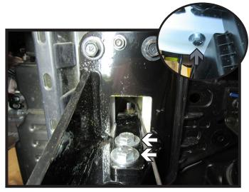
Install 3/8" bolts with flat washers and nylon lock nuts into the front two (2) holes (white). In the back hole install one (1) 1/2" bolt with lock washer, large flat washer, small flat washer from the bottom of the frame and a whiz nut through the frame opening (inset).
