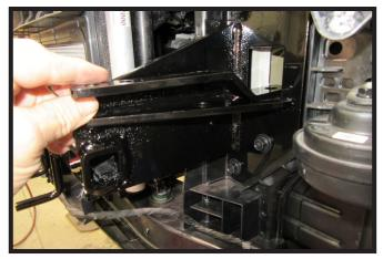
12. Slide frame support brace into place.
