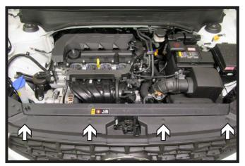
1. Remove the four (4) push pins along the top of the fascia.
