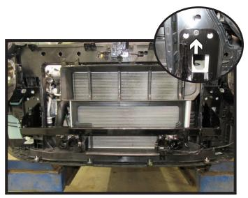
8. Slide the baseplate into place. Install the existing 5MM nut on both sides vehicle to hold the baseplate in place (inset).
