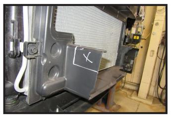
6. Trim the plastic piece on the passenger side of the vehicle as shown.
