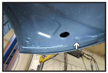
3. On the underside of the vehicle remove the indicated push pin. Do this on both sides of the vehicle.
