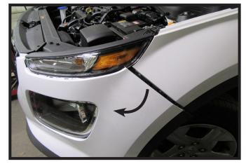
4. Remove the vehicle fascia by pulling upward and outward at the fascia joint to release fascia. Unsnap fascia underneath head light. Do this on both sides of the vehicle. Set fascia aside to be reinstalled later.
