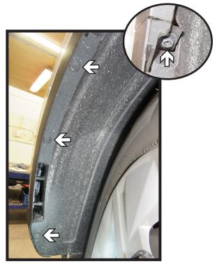
Remove the three (3) push pins along the edge of the wheel well. Then using an 8MM socket, remove the one (1) bolt from the fascia joint (inset). Do this on both sides of the vehicle.
