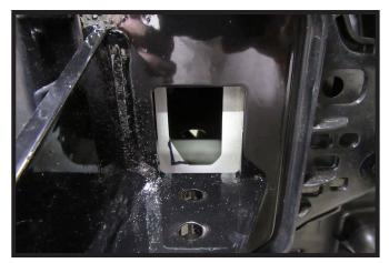
11. Using a reciprocating saw, notch the frame as shown to allow room for the frame support brace. Do this on both sides of the vehicle.
