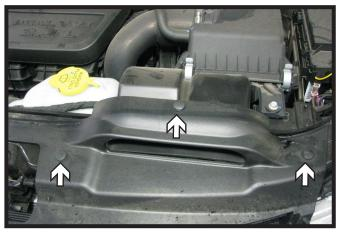
Remove the five (5) push pins from the top of the fascia. Three (3) on the driver side and two (2) on the passenger side.
