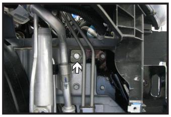
16. On the passenger side, level up the baseplate and clamp to the frame. Using a 13/32" drill bit, drill the upper left hole thru the frame. Install a 3/8"-16 x 1-1/4" bolt and lock washer into hole. From the inside of the frame install a 3/8" flat washer and 3/8"-16 lock nut onto the bolt and tighten. Drill the remaining two (2) holes and install the 3/8" fasteners.
