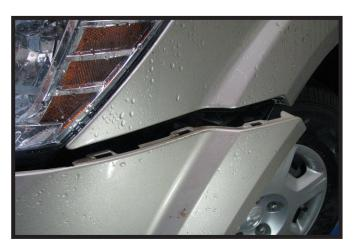
Lift up and pull out on the corners of the fascia to unhook it from the body. Unhook any electrical connections and set fascia aside.
