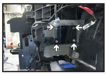
15. Slide the baseplate onto the vehicle. On the driver side, install four (4) 8MM-1.25 x 35MM bolts into the existing holes. Tighten down the bolts but DO NOT use loctite on threads at this time.
