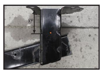
13. On the top side of the bumper, place a mark 3" from the back and centered across. Drill out using a 1-1/4" holesaw. Do this on both sides of the bumper.
