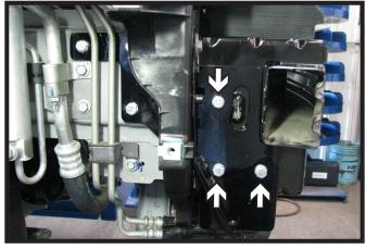
17. Reinstall the bumper onto the vehicle using the existing fasteners. Using a 13/32" drill bit, drill the three (3) holes thru the bumper. Install a 3/8"-16 x 1-1/4" bolt, 3/8" lock washer and 3/8"-16 nut plate into each of the holes using the 1-1/4" hole in the top of the bumper for access. Do this on both sides of the vehicle.
