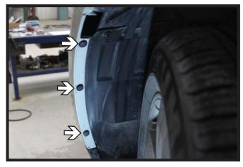
2. Remove the three (3) push pins from the wheel well. Do this on both sides of the vehicle.
