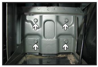
Using a 13MM socket, remove the four (4) bolts from the battery tray. Set the battery tray aside, the bolts will not be reused.
