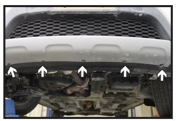
Continue along the underside of the fascia removing the five (5) push pins along the front.
