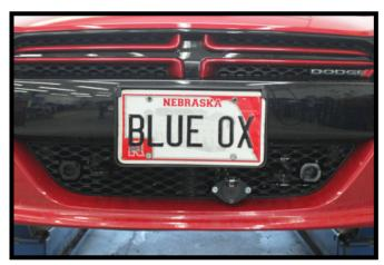
12. Hold the fascia as close to its original position, mark and trim the fascia around the convenience links and attachment tabs. Reinstall the fascia and fascia cover.
