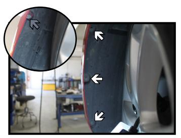
Using a 10MM socket, remove the one (1) upper screw from wheel well (inset). Using a 8MM socket remove the lower three (3) screws from wheel well (white). Do this on both sides of vehicle.
