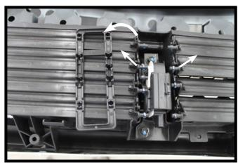
Remove the bracket in the middle of the shutter. Remove the second blade from the top of the shutter on both sides. Then reinstall the bracket.
