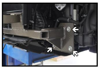
Attach the baseplate to vehicle using the six (6) existing holes and bolts. Be sure to use Loctite<sup>®</sup> Red on threads before tightening.
