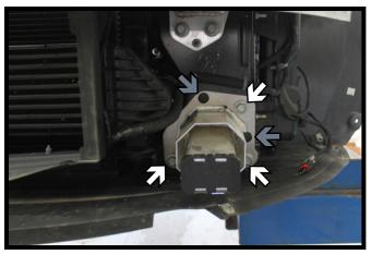
6. Remove the two (2) push pins from the brace (gray). Using a 15MM socket remove the three (3) bolts from brace (white). Do this on both sides of vehicle. Set aside the bolts for installation of baseplate, the brace and push pins will not be reused.
