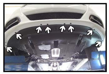
4. Using a 8MM socket remove the eight (8) screws from underneath the fascia.
