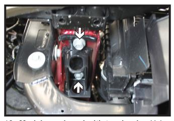
10. **Models equipped with tow hooks:** Using a 16MM socket, remove the two (2) bolts from the tow hook bracket. Remove the tow hook bracket from the vehicle. Do this on both sides of the vehicle.
