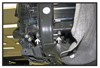
11. **Models equipped with tow hooks:** Slide the baseplate into position on the frame. Install two (2) 10MM-1.5 x 80MM bolts with 10MM lock washers into the bottom holes (white). Install 10MM-1.5 x 100MM bolts with 10MM lock and 3/8" flat washers through the baseplate into the bumper on both the front holes (gray). Tighten all hardware. Do this on both sides of the vehicle.
