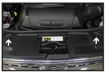
1. Remove the two (2) Phillips head push pins from the top edge of the fascia.
