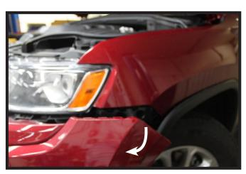
6. Pull the top corners of the fascia out releasing the clips behind, continue working inward towards the grill releasing the clips under the headlights. Pull the fascia forwards disconnecting all electrical connections and set the fascia aside to be reinstalled later.
