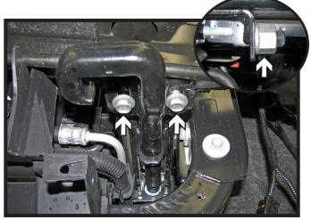
9. **Models equipped with tow hooks:** Using a 16MM socket, remove the two (2) bolts from the front side. Then using a 30MM socket or wrench, remove the nut from the backside of the tow hook. Remove the tow hook from the vehicle. Do this on both sides of the vehicle.
