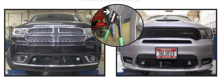
16. Hold the fascia as close to its original position, mark and trim the fascia around the convenience links and attachment tabs. Reinstall the fascia. Using the rivet gun, replace the rivets that were removed during the fascia removal.
