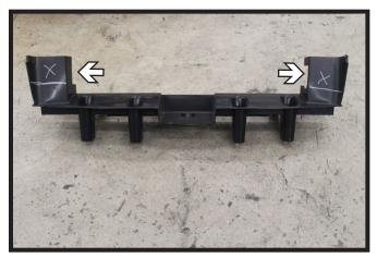
14. Trim the plastic support on the backside of the fascia as shown for baseplate clearance.
