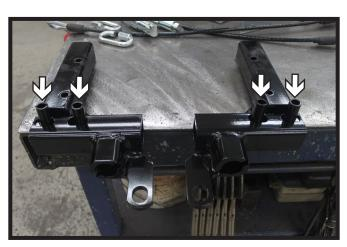
8. Prior to installing the baseplate on the vehicle, install the appropriate spacer tubes into the slots of the baseplate. The tubes will vary depending on whether the vehicle is equipped with tow hooks or not. Reference page 3.
