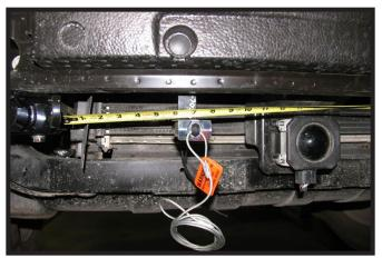
15. **Optional Breakaway:** In the desired location, install the bracket to the bumper with a #10-16 x 1" self drilling screw. Attach the breakaway to the bracket with a 1/4"-20 x 3/4" bolt and 1/4"-20 lock nut.
