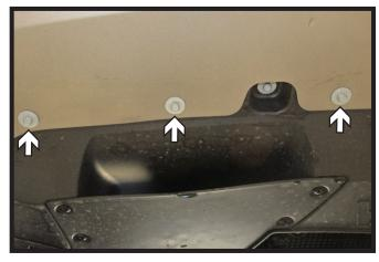
3. **Some Models**: Using a 10MM socket, remove the ten (10) bolts on the underside of the fascia. There are five (5) on each side of the vehicle.
