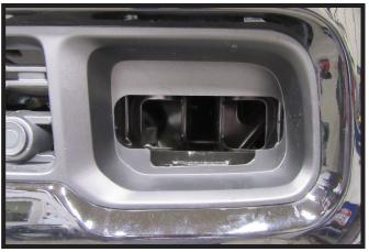
4. Remove baseplate. Using a utility knife trim the marked plastic area. Do this on both sides of the vehicle.
