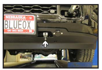
8. **Optional Breakaway**: Using the provided 1/4" hardware, attach the breakaway switch to the vehicle bumper as indicated.
