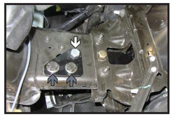
6. Place spacer brackets on both sides of the frame as shown. Install one (1) 5/8" x 4-1/2" bolt (white). Then install the two (2) existing 16MM bolts (gray). Tighten all bolts fully. Do this on both sides of the vehicle.
